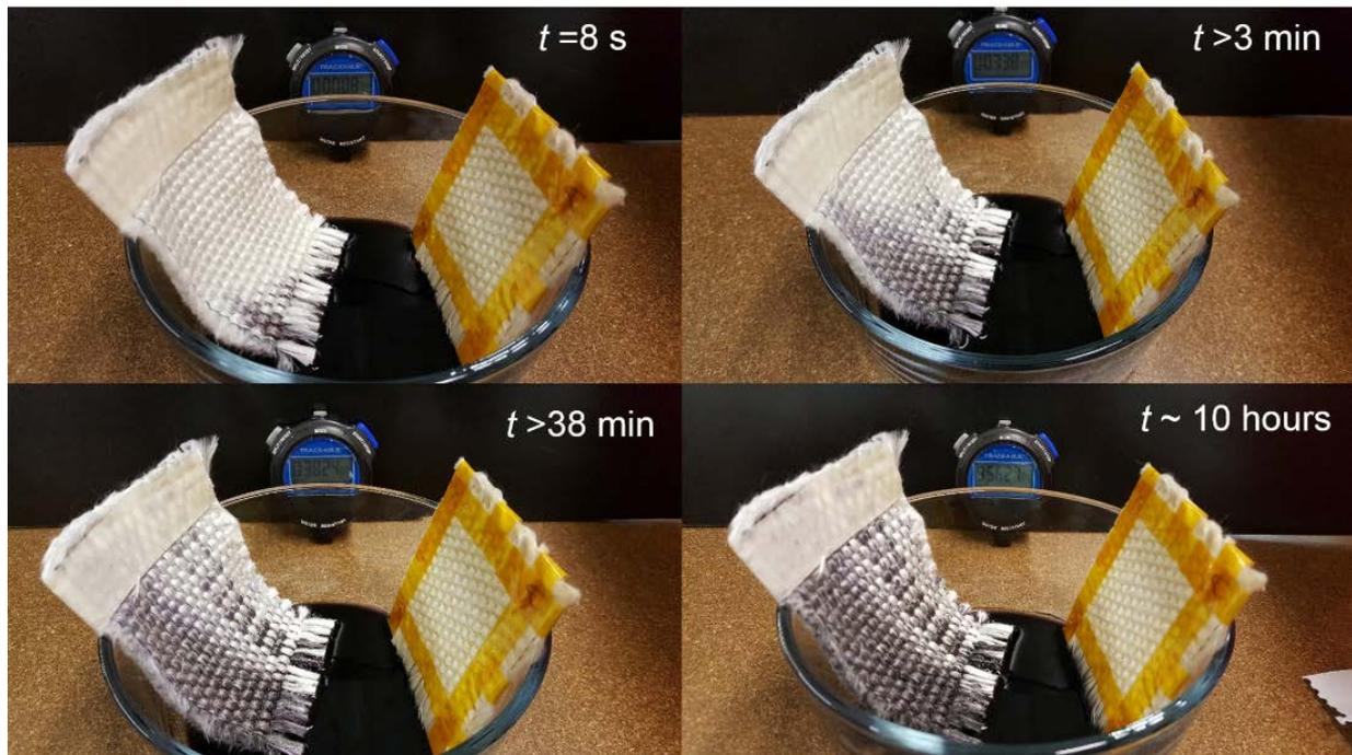
Fig. 3. Wicking test using a dye water at different times. Times (indicated by  $t$ ) are shown at the top right of individual picture. The cloths at the left and right sides of the bowl correspond to the uncoated and ALD-coated cloths, respectively.
