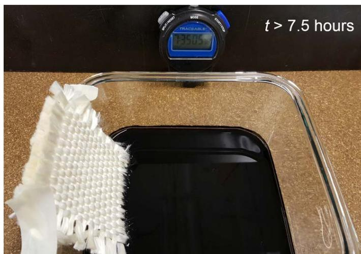
Fig. 4. Wicking test after heating the ALD-coated fiber cloth up to 200°C for one hour. The wicking test was performed for over 7.5 hours.
