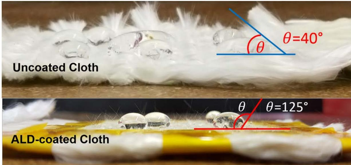
Fig. 2. Water droplet formation on the uncoated and ALD-coated fiber cloths.
