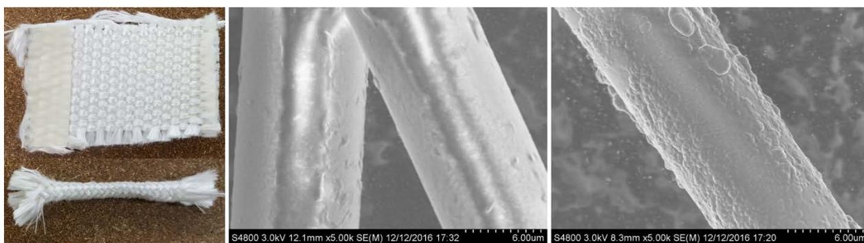
Fig. 1. [Left]: flat and sleeving glass fiber cloths at top and bottom of the picture, respectively. [Middle]: SEM image of uncoated cloth. [Right]: SEM image of ALD-coated cloth with 200 nm  $\text{Al}_2\text{O}_3$  films.
