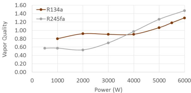
Figure 7. Comparison of the vapor quality leaving the evaporator as a function of input power
