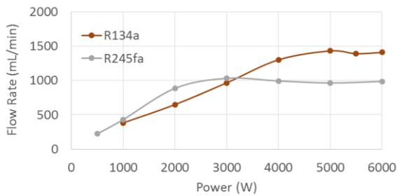
Figure 6. Comparison of fluid flow rate as a function of power for R134a and R245fa
