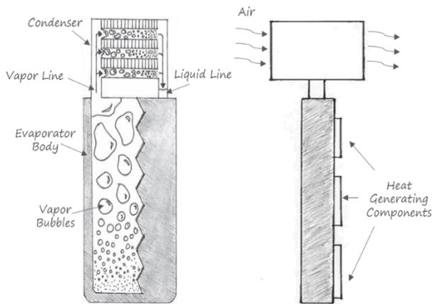
Figure 2. Example of a Loop Thermosyphon for power electronics cooling applications
