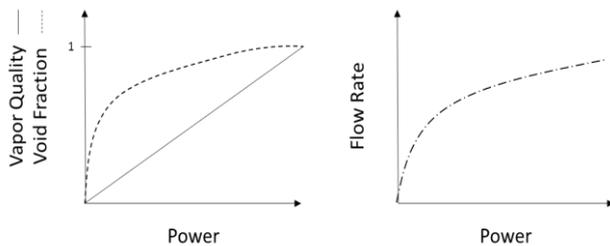
Figure 3. (left) void fraction can be highly non-linear with increasing power while quality remains mostly linear. (right) flow rate in the system is mostly tied to void fraction and behaves similarly with respect to increasing power
