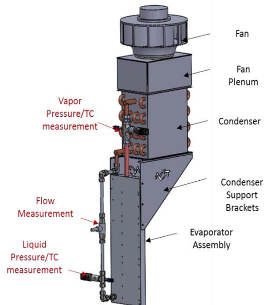
Figure 4. 3D rendering of the experimental apparatus illustrating instrumentation locations from aluminum and instrumented with a turbine flowmeter, temperature and pressure sensors. The evaporator was attached to a standard
