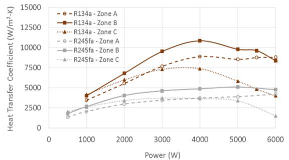
Figure 8. Heat transfer coefficients as a function of power are shown for the various heating zones in the evaporator
