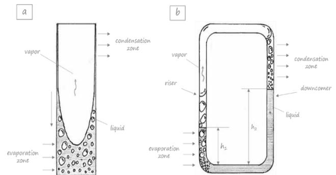
Figure 1. Schematic representation of a (a) traditional Thermosyphon and a (b) Loop Thermosyphon
