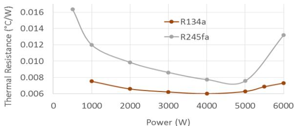
Figure 9. Comparison of the thermal resistance vs input power for R134a and R245fa
