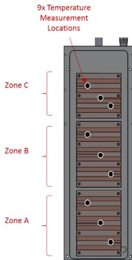
Figure 5. An illustration indicating the locations of heater temperature measurements.
