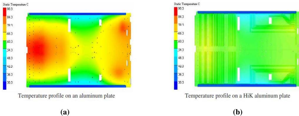
Figure 5. FEA for a particular application with multiple heat sources across the plate. For a) Temperature distribution on the standard aluminum plate b) Temperature distribution on the HiK™ plate. A reduction in peak temperature of 21°C can be observed.
