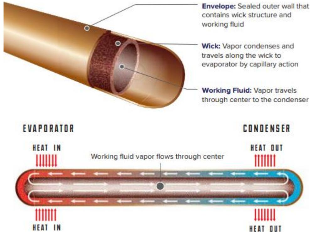
Figure 1. Copper–water heat pipe operation.
