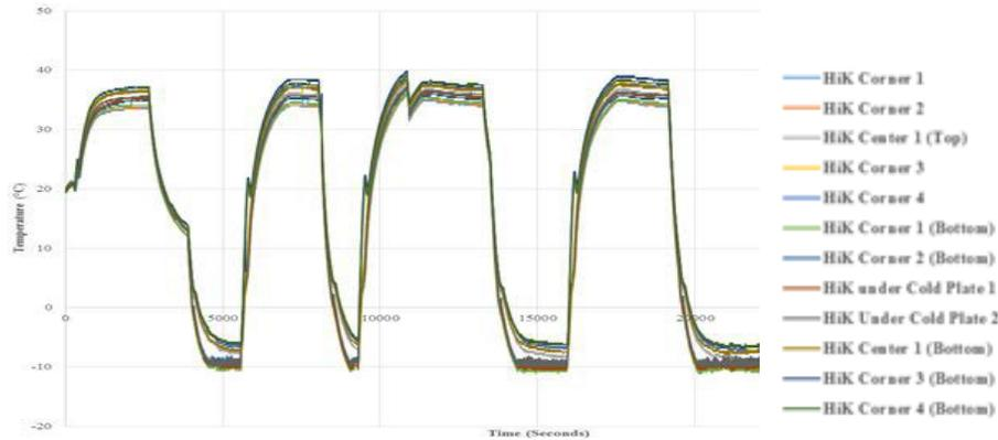
**Figure 10. Snapshot of the temperature profile of HiK™ plate exposed to thermal cycling in orbit.**
