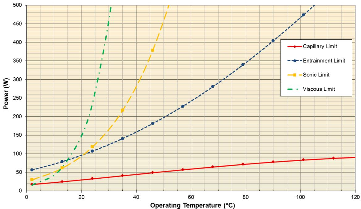
**Figure 6. Heat pipe limit chart for the embedded copper/water heat pipes into the HiK™ plate for ISS APT<sub>x</sub> experiment.**
