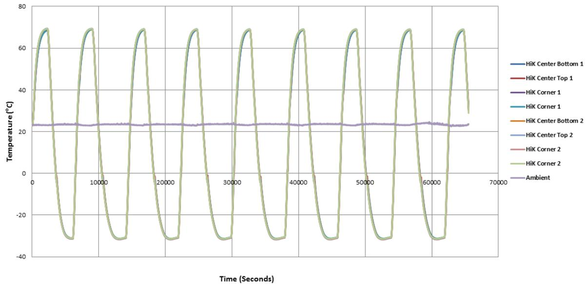
Figure 8. The temperature profile of HiK™ plates exposed to thermal cycling.
