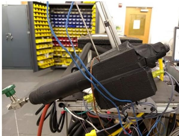
**Figure 7. LHP prototype with flexible lines added to allow for tilting of the evaporator at angles up to 25°**
