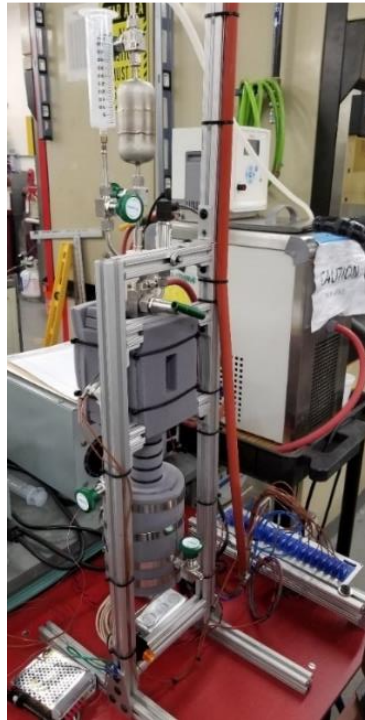
Figure 5: Actual test setup used in the lab to measure the thermal performance of condenser surfaces.
