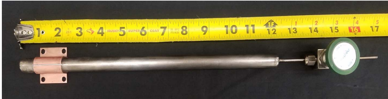
Figure 4. Picture of the High-Heat-Flux Titanium-Water CCHP
