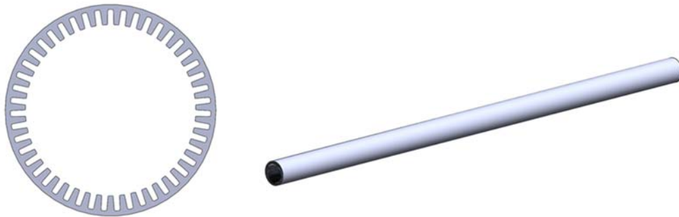
Figure 2. Rendering of the Groove Geometry and Grooved Section of the CCHP Prototypes
