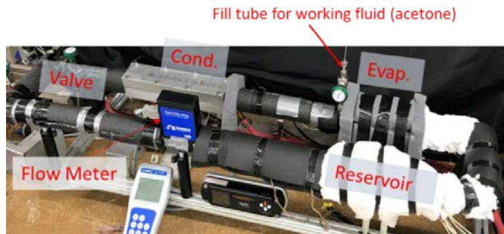
**Figure 11. Experimental apparatus of the VCHP loop concept demonstration**
