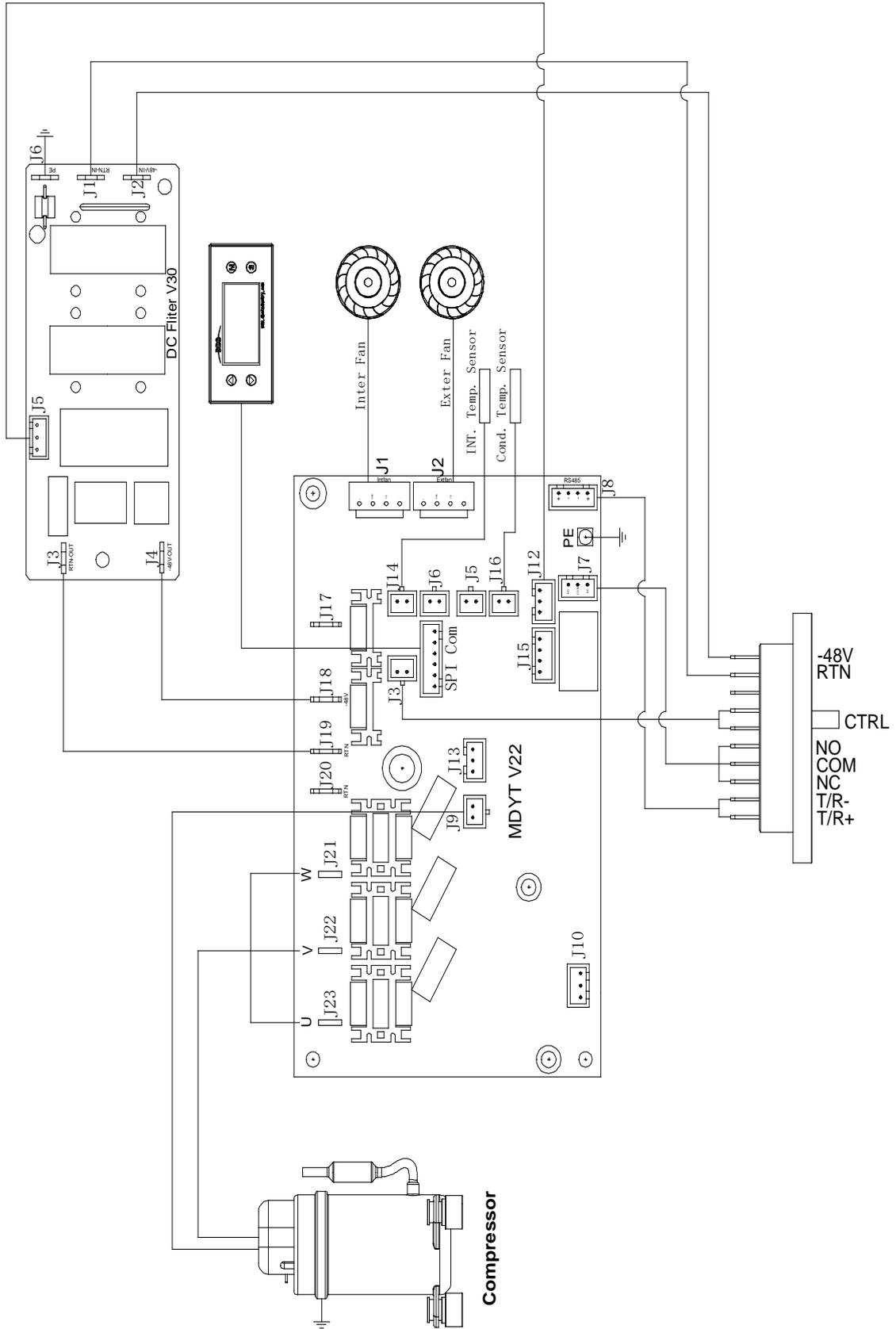
Figure 5.7 System wiring diagram for the **ACT-VCC-3000-DC**
