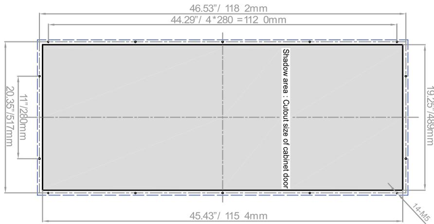
Figure 5.4 Dimensions for cut-out in enclosure door for the **ACT-VCC-2000-AC**
