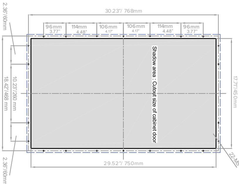
Figure 5.5 Dimensions for cut-out in enclosure door for the **ACT-VCC-5000-AC**
