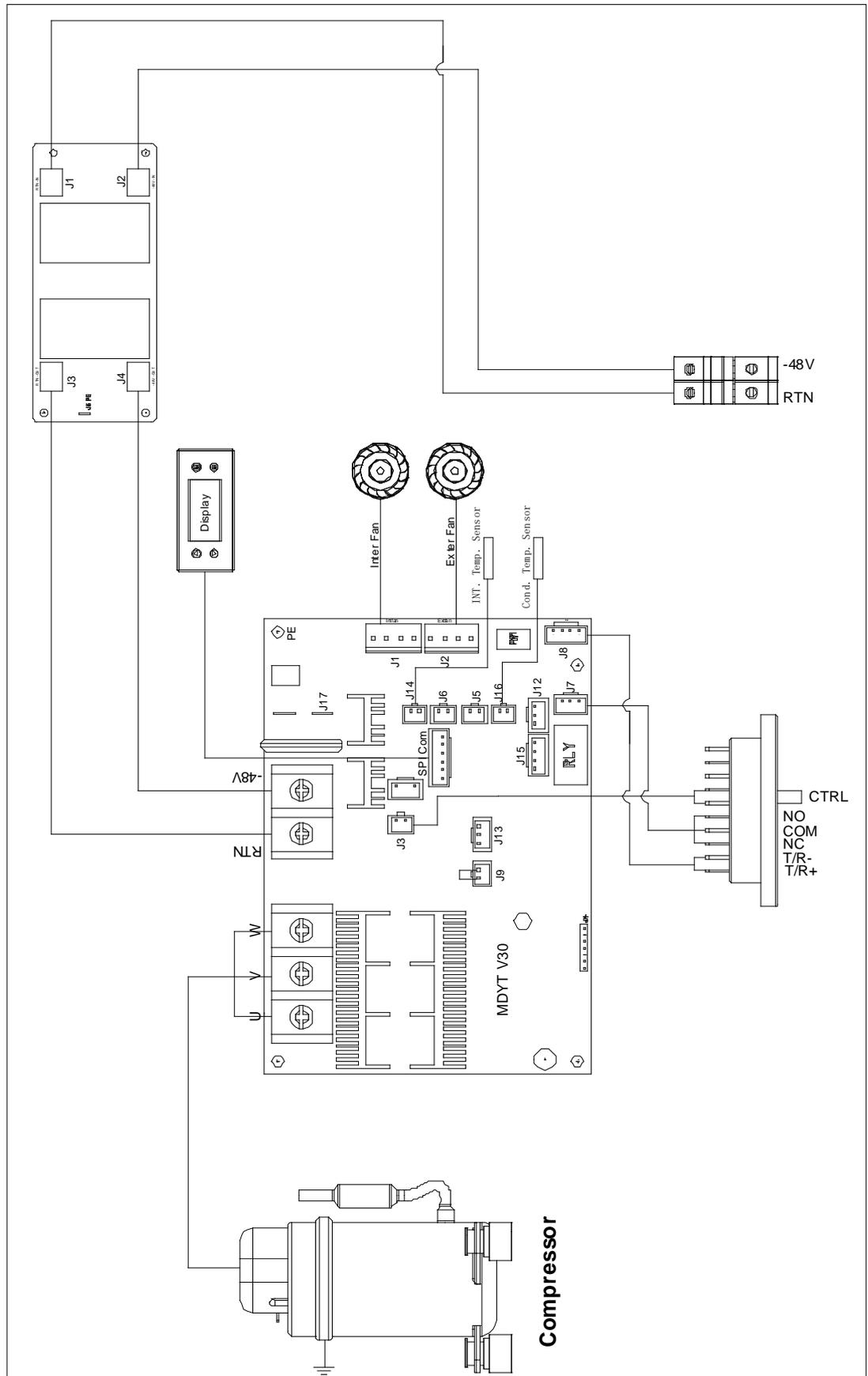
Figure 5.8 System wiring diagram for the **ACT-VCC-2000-AC**
