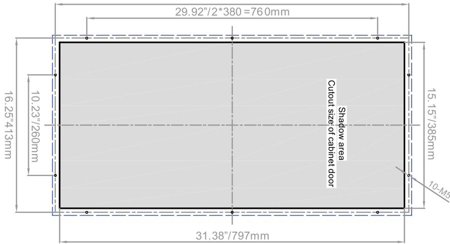
Figure 5.3 Dimensions for cut-out in enclosure door for the **ACT-VCC-3000-DC**
