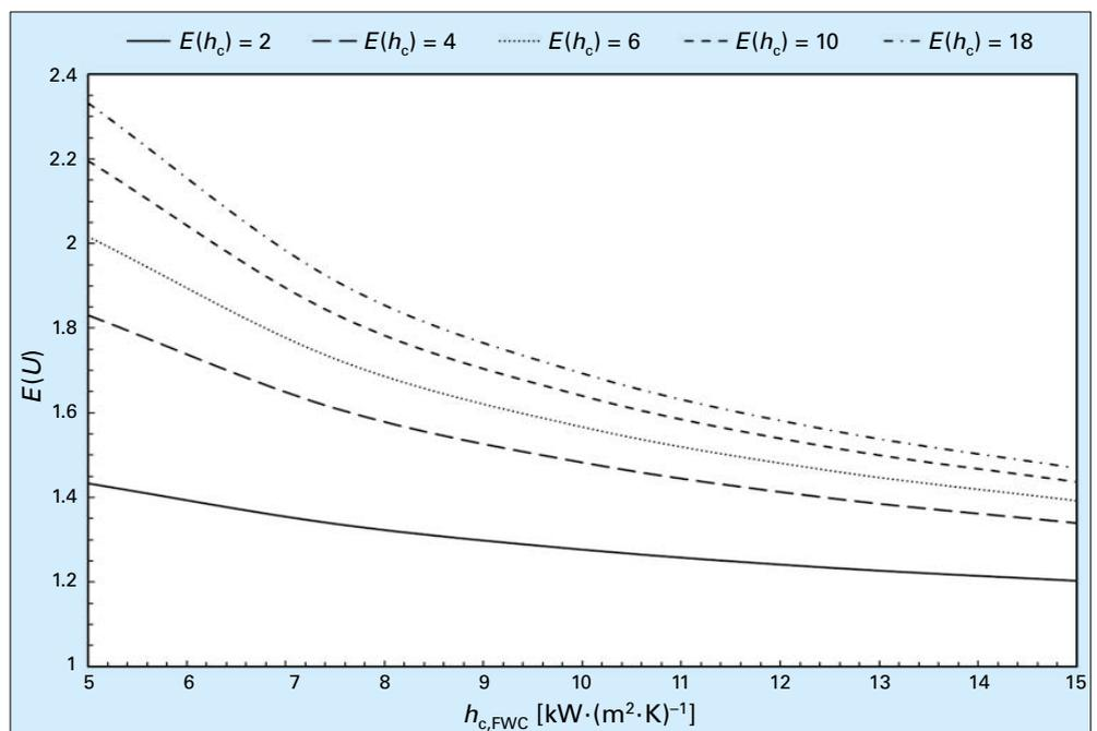
Figure 7: Modeling results for the enhancement in the overall heat transfer coefficient,  $U$ , as a function of the filmwise condensation heat transfer coefficient,  $h_{c,FWC}$ . With a known experimental enhancement in  $h_c$  determined for a steam surface condenser, the range of improvement in  $U$  can be quickly determined as a function of  $h_{c,FWC}$ .
