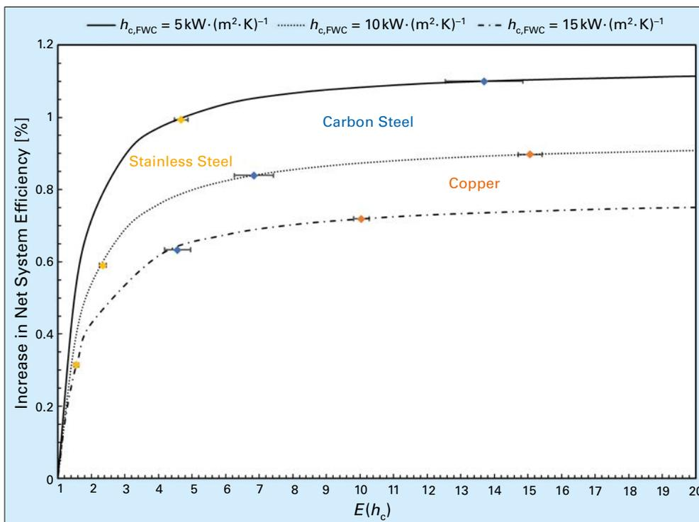
Figure 8: Increase in net system efficiency as a function of the enhancement ratio of the condensation heat transfer coefficient. The font color for each condenser material corresponds with the accompanying data points of the same color.
