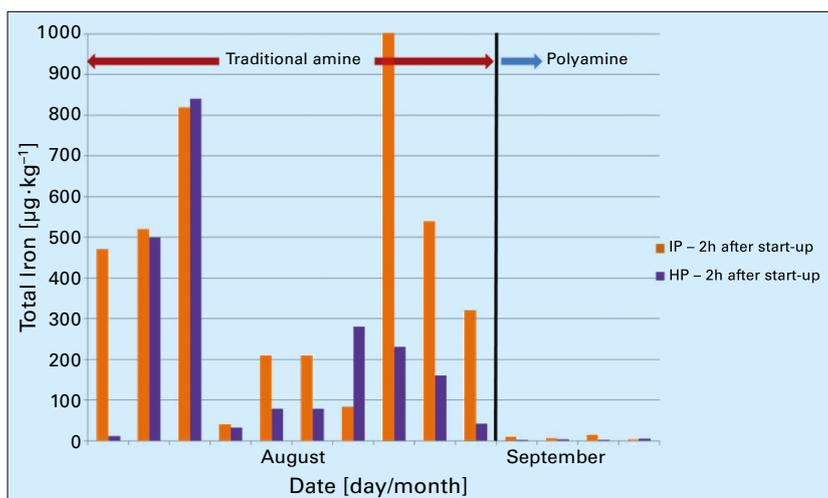
Figure 3: Reduction in iron concentration in the intermediate-pressure (IP) and high-pressure (HP) sections of the HRSG unit of an 850MW combined-cycle plant due to polyamine treatment. There was a 10- to 100-fold reduction in iron transport during continuous steady-state operation and start-ups, respectively (data not shown) [12].
