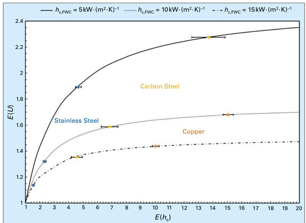
Figure 6: Enhancement ratio of the overall heat transfer coefficient,  $U$ , as a function of the enhancement ratio of the condensation heat transfer coefficient,  $h_c$ . The data points represent the experimental enhancement of  $h_c$  superimposed on the results for the modeling curves. The font color for each condenser material corresponds with the accompanying data points of the same color.
