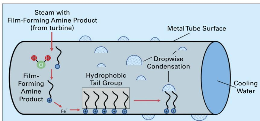
Figure 4: Detailed configuration of FFAP coating applied to a steam surface condenser tube.
