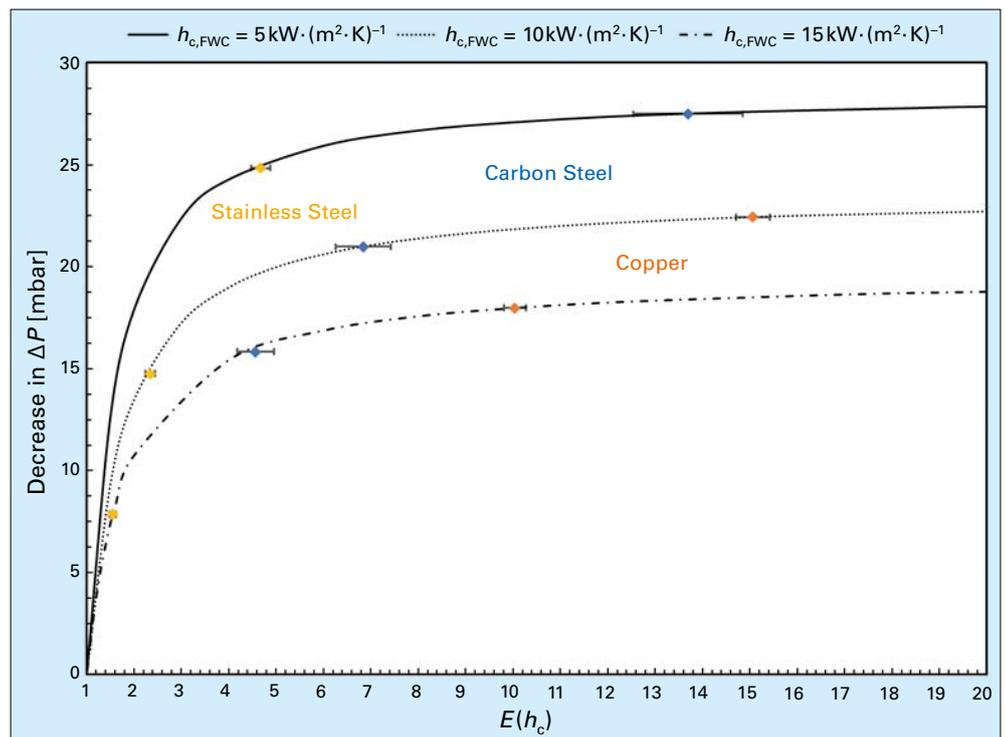
Figure 10: Decrease in turbine backpressure as a function of the enhancement ratio of the condensation heat transfer coefficient. The font color for each condenser material corresponds with the accompanying data points of the same color.
