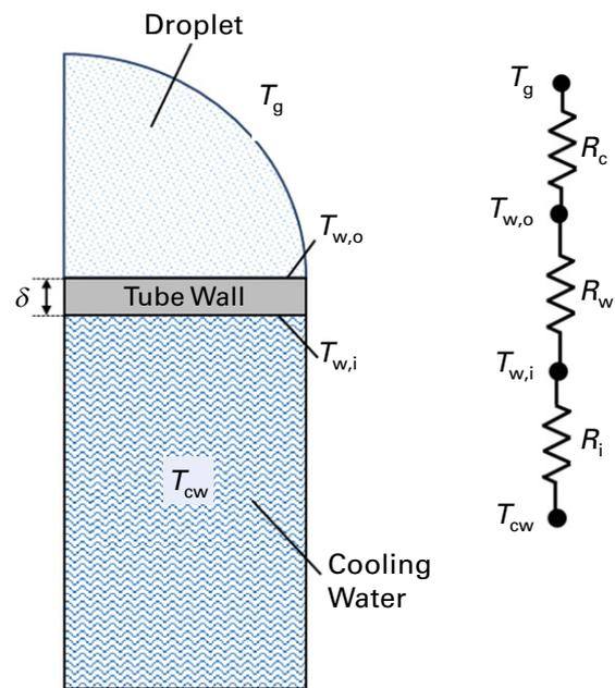
Figure 5: 1-dimensional representation of the demonstrated thermal resistance network model for saturated steam,  $T_g$ , condensing on a portion of the tube wall on the shell-side, with heat removal due to cooling water,  $T_{cw}$ , on the tube-side.
