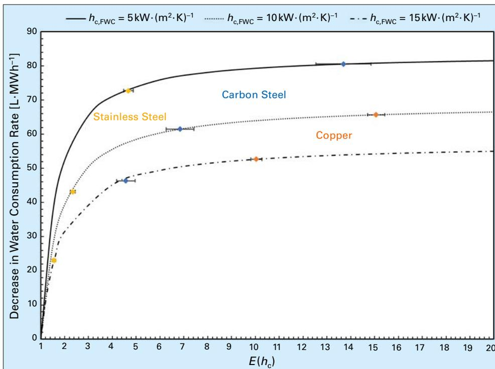
Figure 9: Decrease in water consumption rate as a function of the enhancement ratio of the condensation heat transfer coefficient. The font color for each condenser material corresponds with the accompanying data points of the same color.
