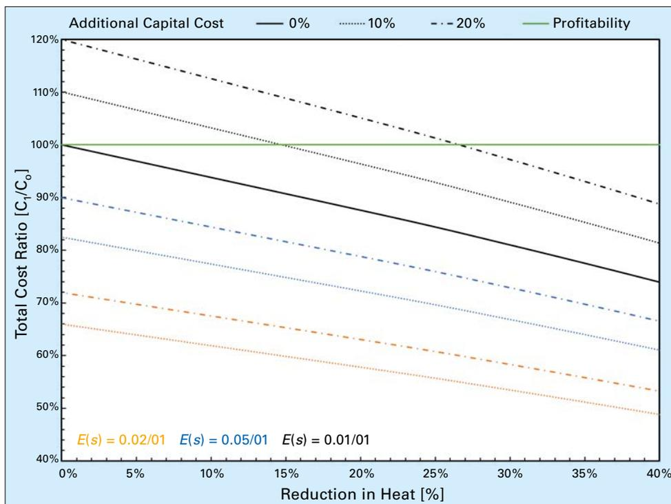
Figure 12: The total cost ratio as a function of the reduction in tubing heat transfer surface area for different maintenance cost ratios and additional capital cost requirements. Any value below the profitability line is a profitable scenario.
