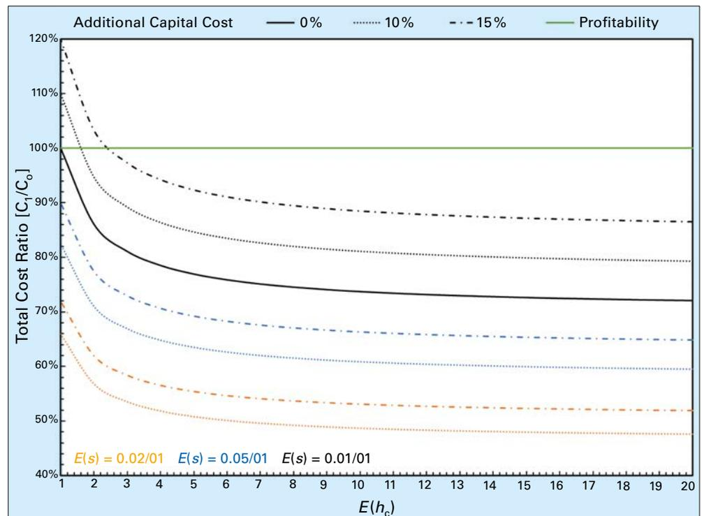
Figure 11: The total cost ratio as a function of the enhancement of the condensation heat transfer coefficient for different maintenance cost ratios and additional capital cost requirements. Any value below the profitability line is a profitable scenario.
