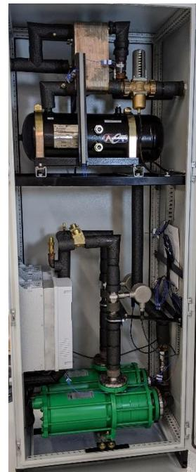
**Fig. 8:** Thermal cabinet with balance of plant components
