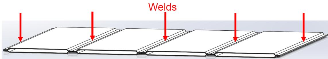
Figure 6. Welding pattern for multi-channel VVFTPR
