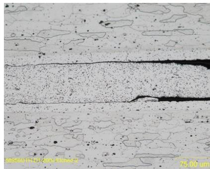
**d) 0.020 in. thick with .002 in. thick interlayer. Cracking at edge extending into weld.**
