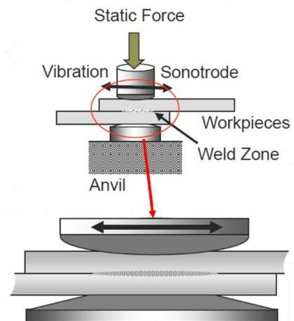
Figure 5. Illustration of the ultrasonic welding process. Source EWI.
