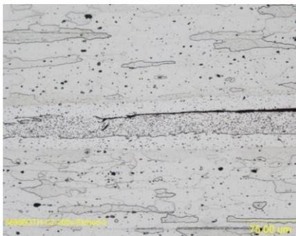
**c) 0.020 in. thick with .001 in. thick interlayer. Cracking at edge extending into weld.**
