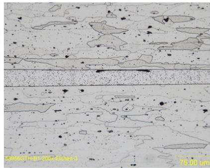
**b) 0.012 in. thick with 0.002 in. thick interlayer. Gap between top sheet and interlayer.**
