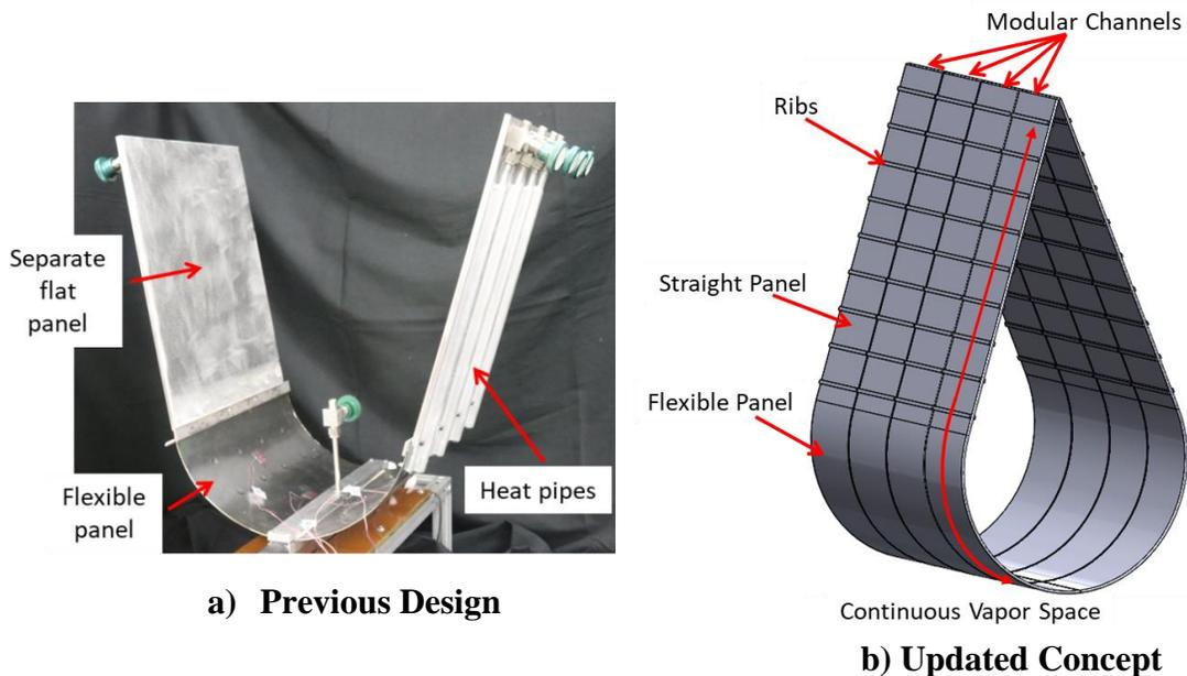
**Figure 2. Overview of the variable-view factor two-phase radiator concept evolution: (a) previous design, (b) updated second-generation design.**
