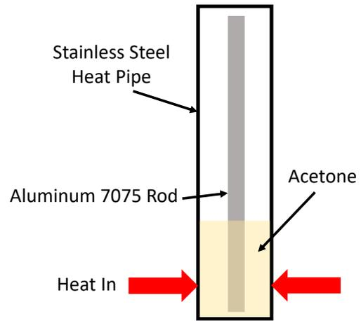
Figure 4. Illustration of compatibility test between acetone and aluminum 7075.
