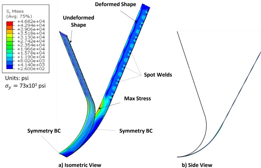
**Figure 9. Simulations results of single channel prototype. Aluminum 7075. Wall thickness 0.012 in. (0.305mm), channel width 1.5 in. (38.1 mm). Internal pressure was 11.82 psi which corresponds to acetone saturation pressure at 50°C.**
