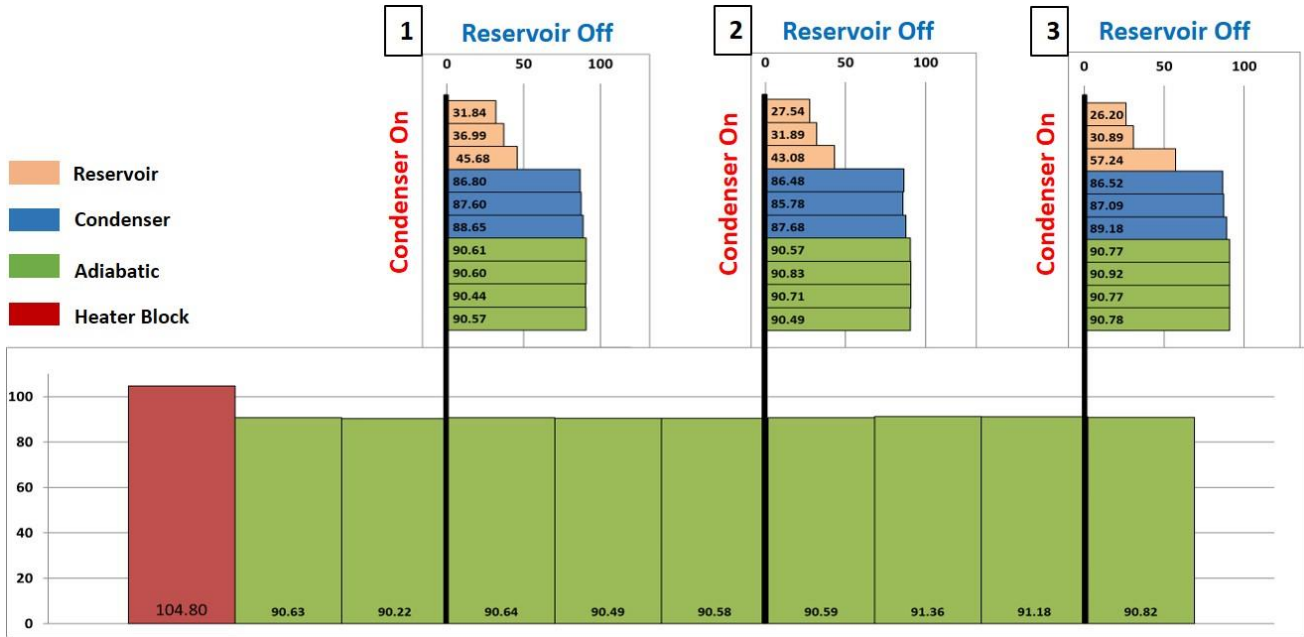
Fig. 9 Temperature distribution of MVCHP when all reservoirs are unheated. All condensers are fully open.
