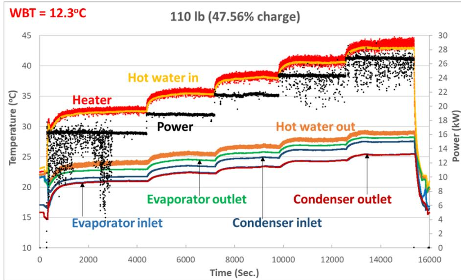
Figure 12. 110 lb charge test data.
