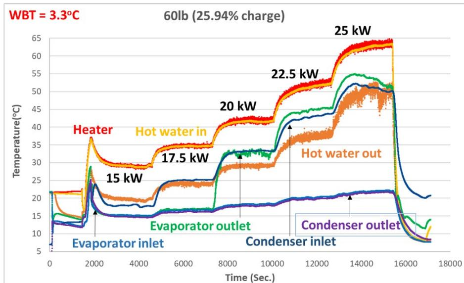
*Figure 7. 60 lb charge test data.*
