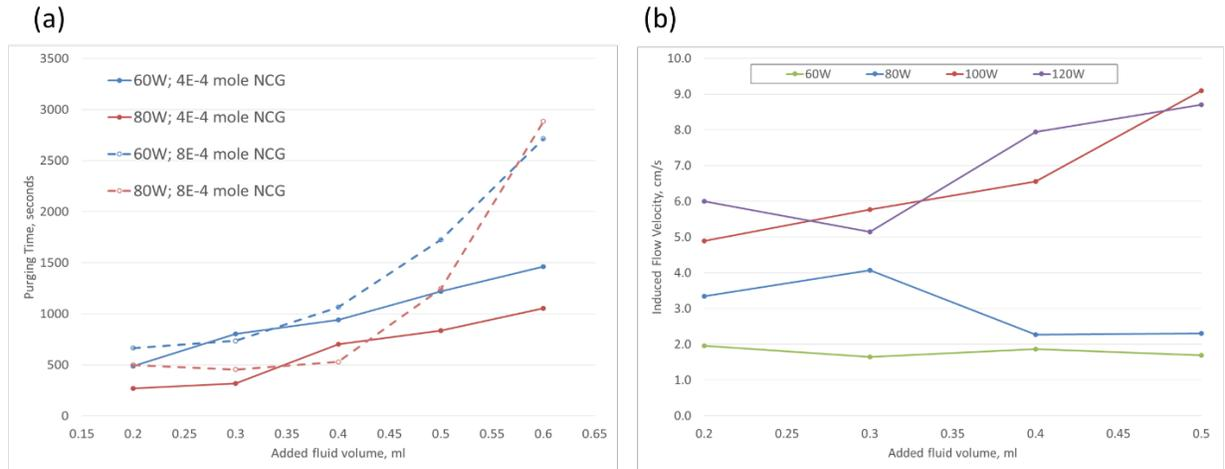
Figure 13. (a) Measured purging time with different heating powers and NCG amount (b) estimated bulk momentum-induced flow velocity under different heating powers with NCG of  $4 \times 10^{-4}$  moles.
