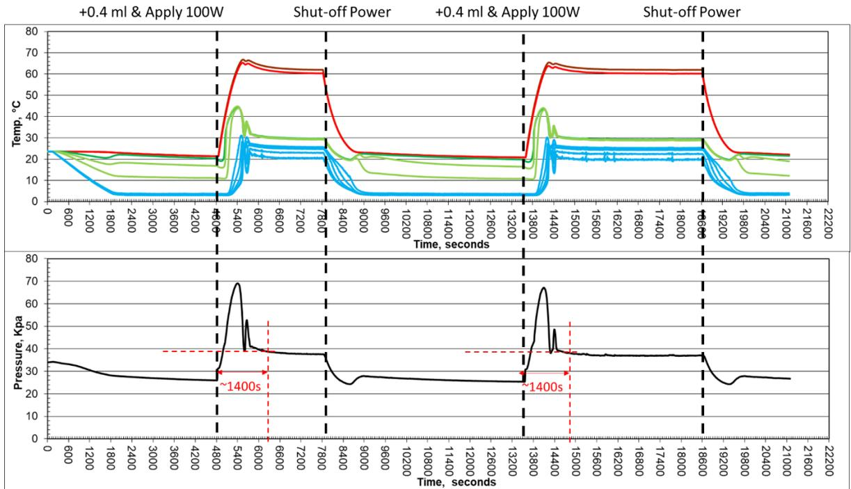
**Figure 15. Startup of VCHP Loop from 100% humidity reservoir (conservative scenario).**
