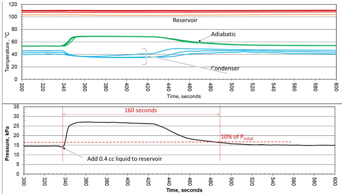
**Figure 14. Purging test results with toluene as working fluid and helium as NCG.**
