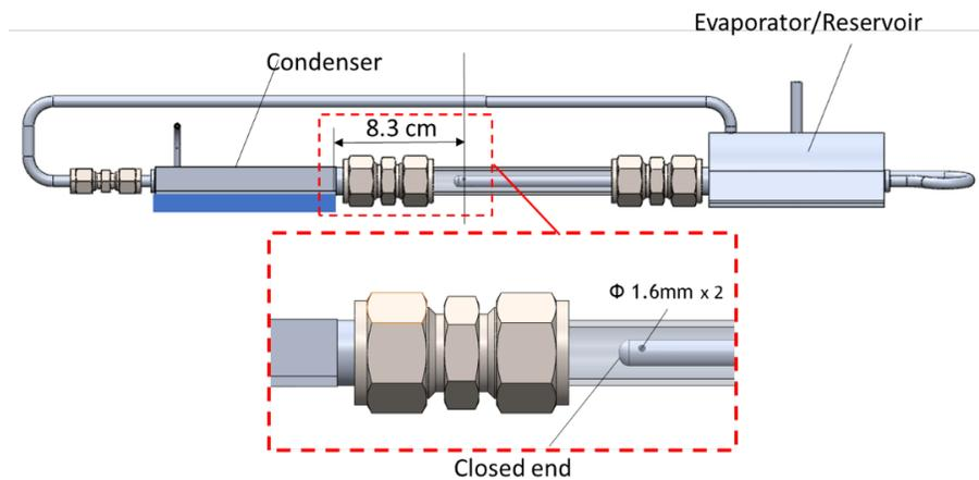
**Figure 3. CAD of VCHP loop and detailed drawing of internal NCG tube design (two-hole Venturi style).**
