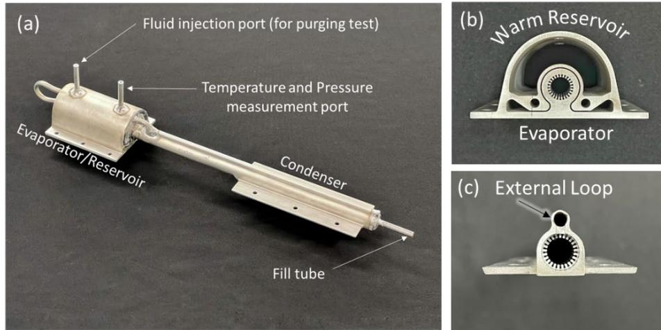
**Figure 17. A compact VCHP loop with both reservoir and external loop integrated (a) isometric view (b) reservoir integrating with the evaporator (c) external NCG tube integrated with the heat pipe section.**
