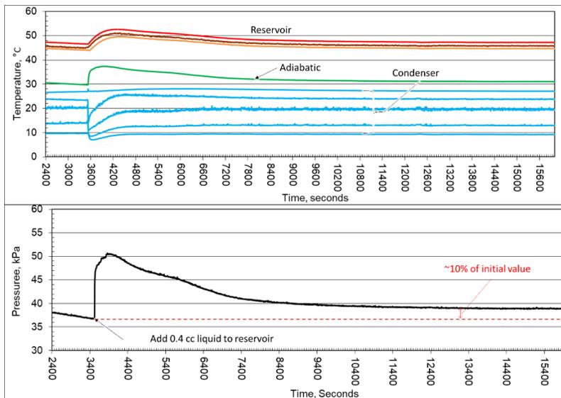
Figure 6. Purging test results of VCHP without a loop. The top figure shows the temperature variation and the bottom figure shows the pressure variation.
