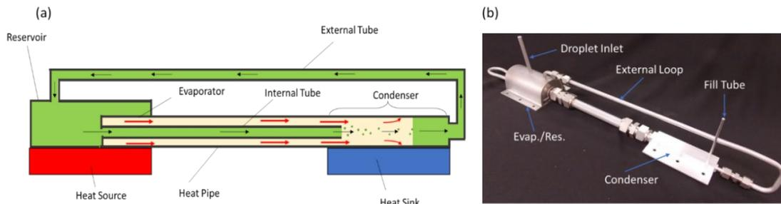
**Figure 1. Advanced hot reservoir VCHP with (a) conceptual design of VCHP (b) proof-of-concept prototype developed in Phase I.**
