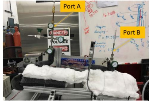
Figure 5. Experimental system for VCHP purging test.
