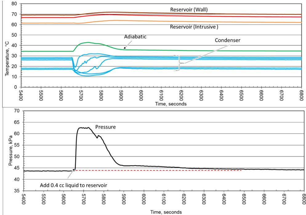
**Figure 7. Purging test results of VCHP loop. Top: Temperature variation; Bottom: Pressure variation.**
