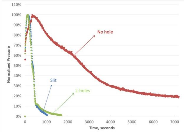
**Figure 9. Purging rate with different NCG tube designs.**
