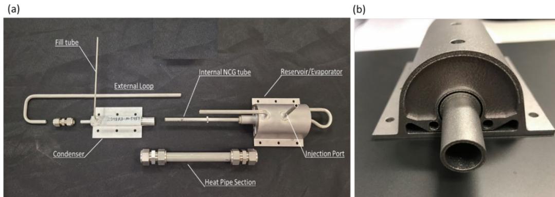
**Figure 2. Aluminum VCHP loop prototype with an integrated reservoir (a) all components (b) additive manufactured evaporator/reservoir.**
