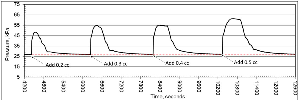
**Figure 8. Repeatability test of VCHP loop purging (2-hole outlet).**
