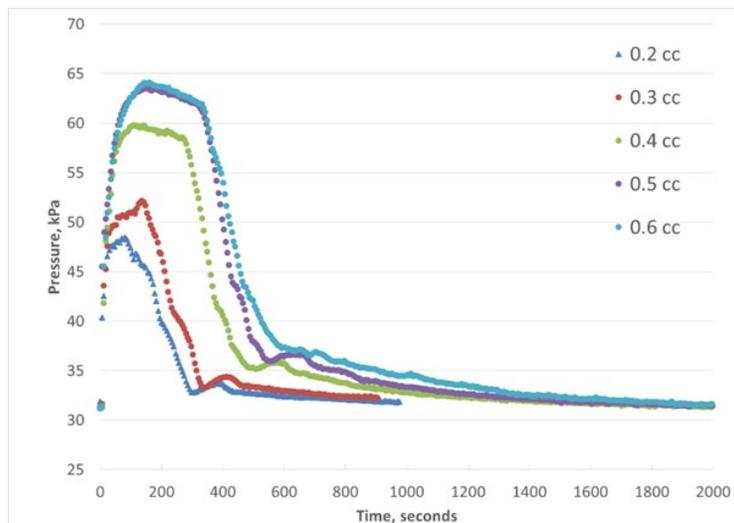
Figure 12. Purging rate with different added fluid volume into a warm reservoir.
