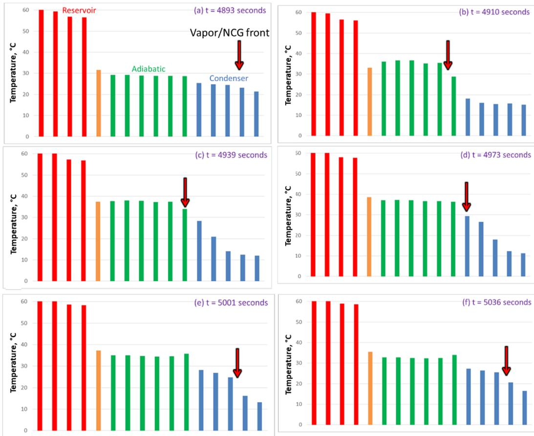
Figure 11. Instantaneous temperature profiles at different time stamps during purging (red arrow indicates the vapor/NCG front location).
