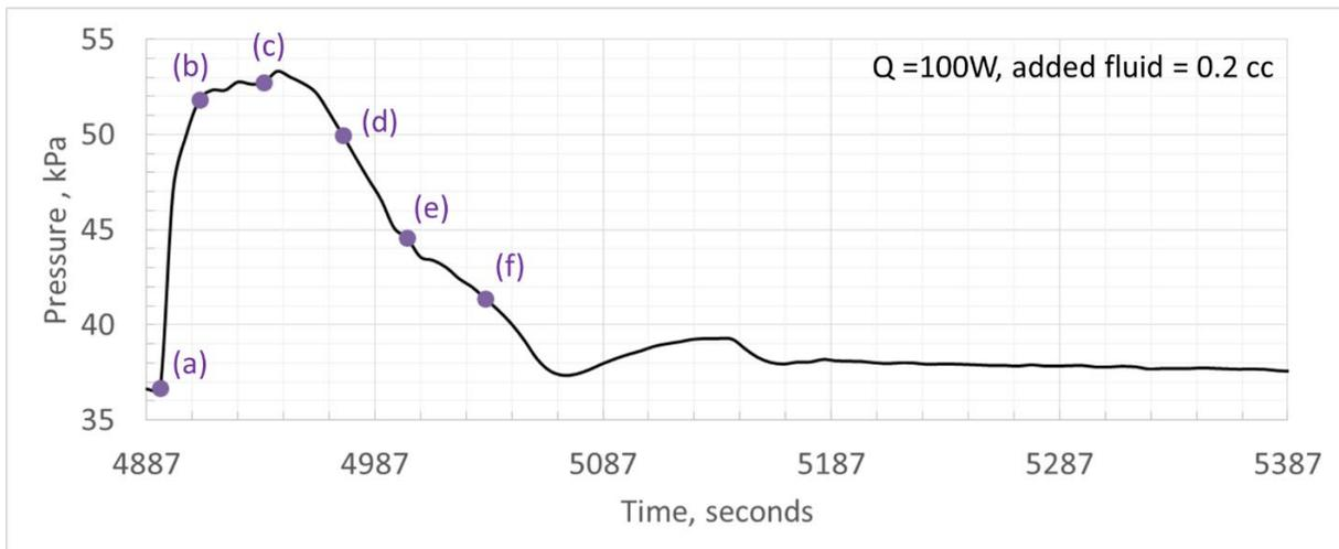
**Figure 10. Pressure variation during purging. Heat input of 100W; 2-hole NCG tube design; added acetone liquid = 0.2 cc to the reservoir.**
