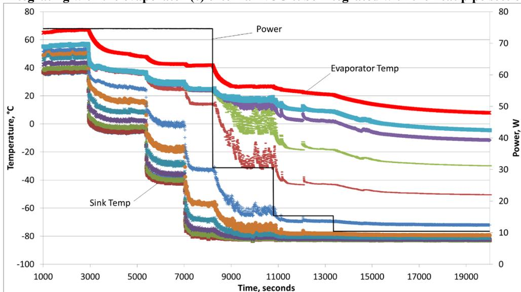
**Figure 18. Thermal control performance of the VCHP loop.**
