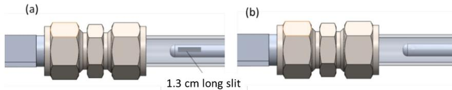
**Figure 4. (a) Slit NCG tube (b) fully-closed NCG tube.**
