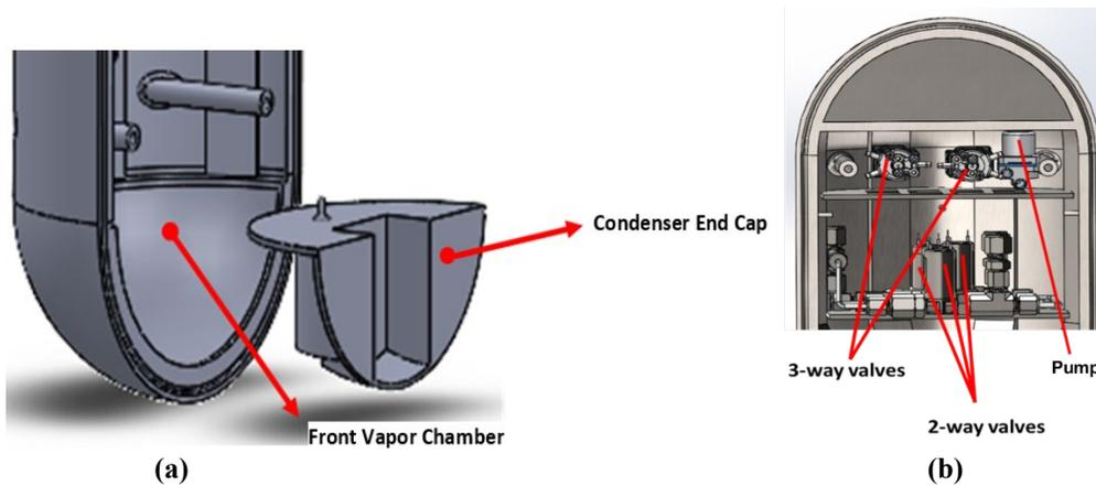
**Figure 4: (a) Front vapor chamber space at the bottom of ACT's melting probe prototype (b) Liquid Displacement System (LDS) at the top of the melting probe prototype.**
