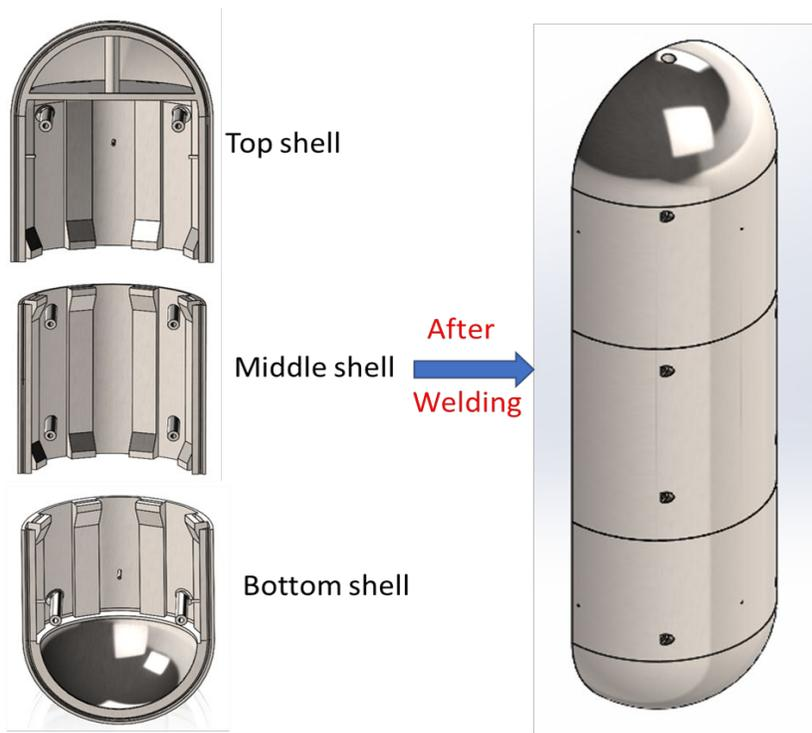
**Figure 5: Shell components for fabrication of ice melting probe before and after welding.**
