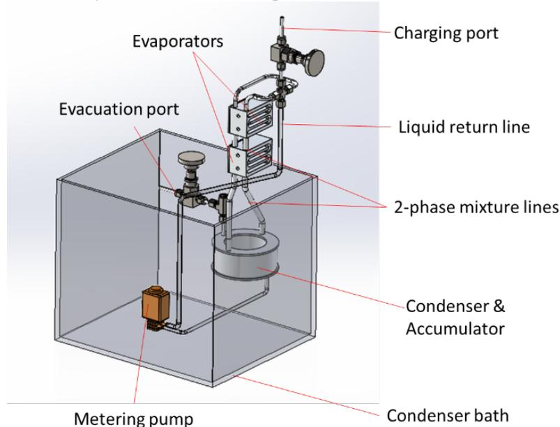
Figure 6: P2P loop with mixed two-phase flow evaporators for 800 W of heat supply.
