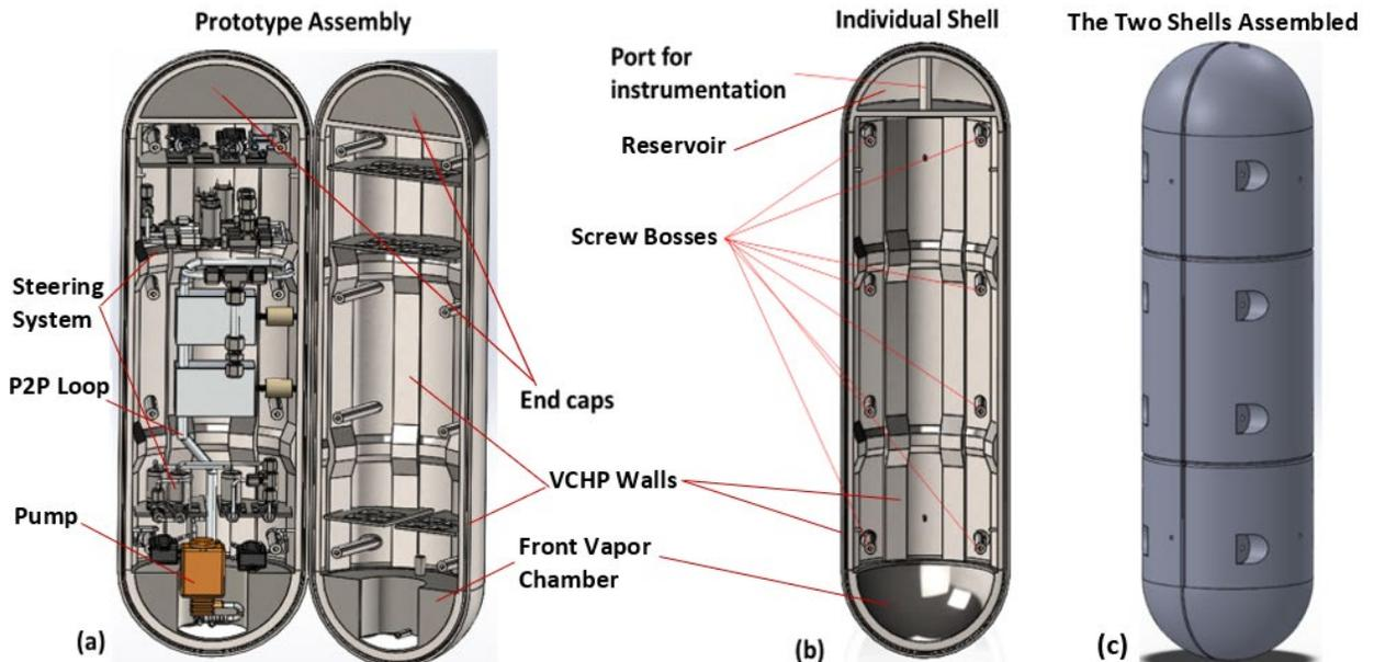
Figure 2: (a) Inside view - CAD model of the full melting probe prototype with P2P loop, front vapor chamber, VCHP walls and liquid displacement (steering) system (b) Inside view of one shell - screw bosses, instrumentation port and VCHP wall are visible (c) Outside view - melting probe prototype with the two shells closed and sealed with a gasket.
