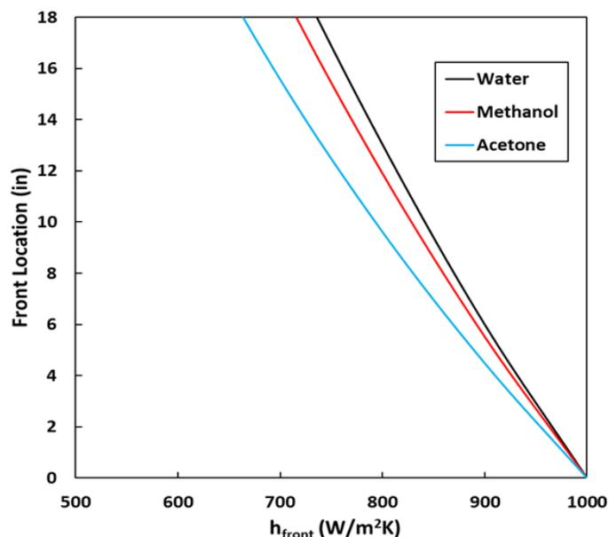
Figure 13: Sensitivity of the vapor-NCG front location for different working fluids for decrease in the front liquid film heat transfer coefficient.
