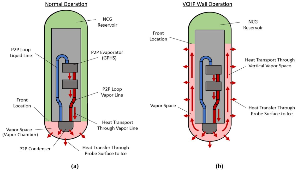
Figure 1: (a) Heat map during normal operating mode with vapor contained in the front vapor chamber and (b) active VCHP wall operating mode with vapor pushing the NCG front up towards the reservoir.
