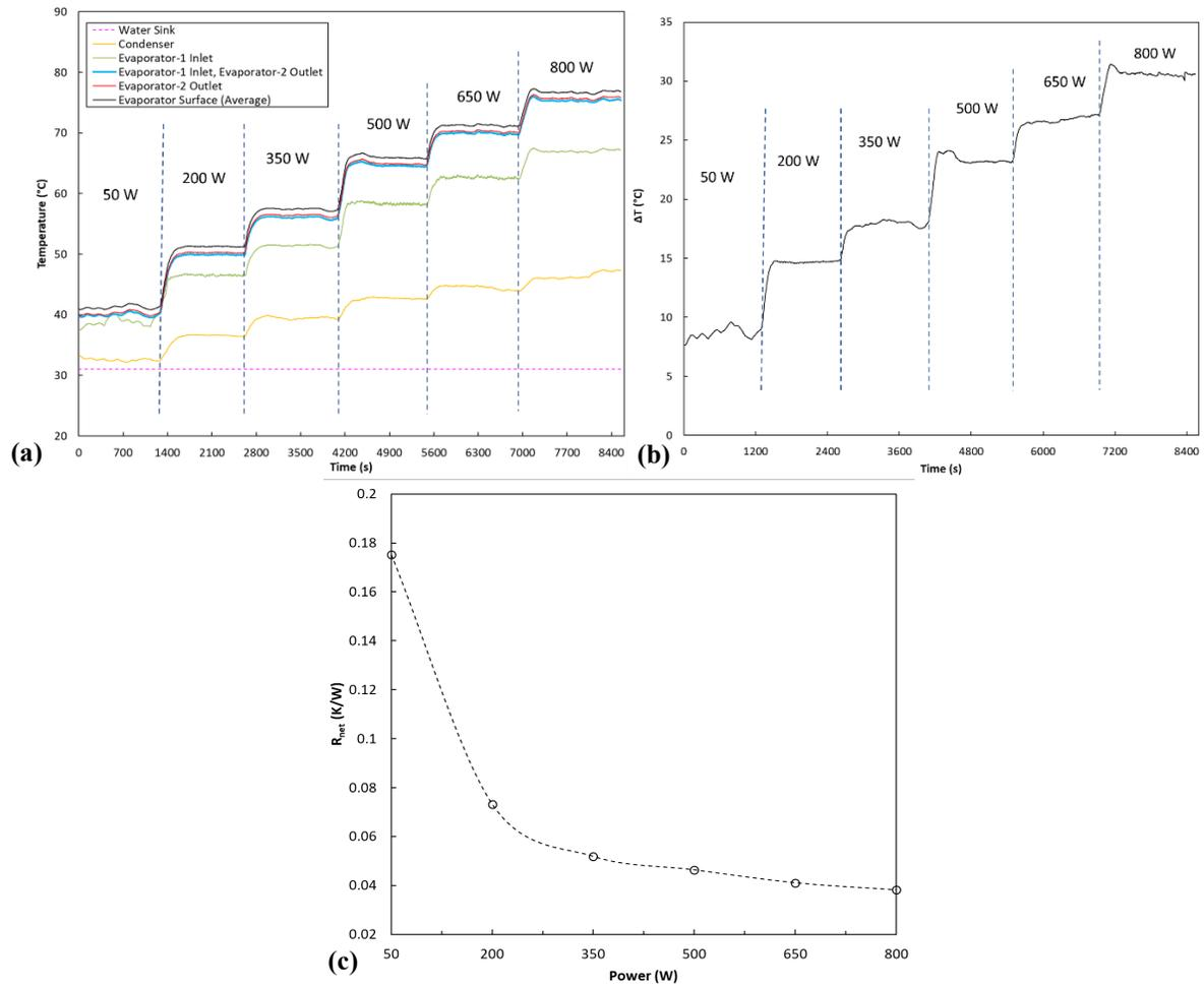
**Figure 9: (a) Temperature measurements for P2P loop for power levels from 50 to 800 Watts with constant volumetric flow rate of 0.6 liters/minute corresponding to 800 Watts power, (b) P2P loop temperature drop  $\Delta T$  (°C) for power levels from 50 to 800 Watts, (c) Thermal resistance  $R_{net}$ (K/W) of P2P loop for power levels from 50 to 800 Watts.**
