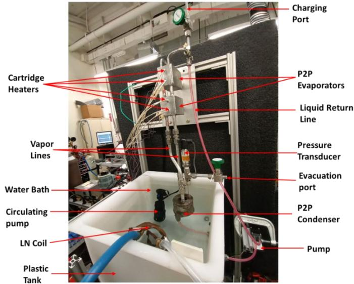
**Figure 8: Experimental setup of P2P loop used for thermal performance testing at ACT.**
