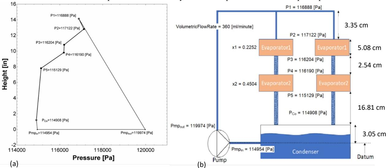
**Figure 7: (a) Two-phase pressures drop plot and (b) schematic of the pressure distribution within the 3<sup>rd</sup> iteration of the P2P loop setup.**
