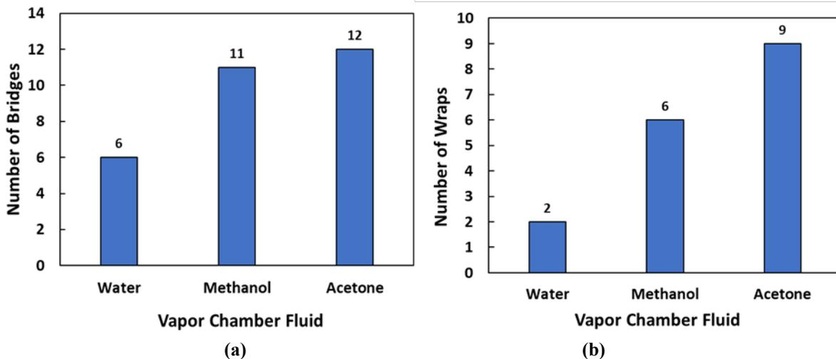
Figure 12: Parametric study of number of bridges (a) and wraps (b) required to transfer 1kW of heat for ACT' ice melting probe prototype.
