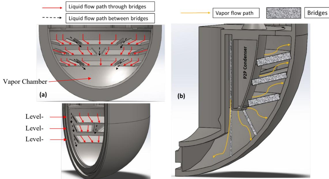
**Figure 11: (a) Liquid flow path through and between the bridges within one of the two vapor chamber volumes, (b) Vapor flow path inside one of the two vapor chamber volumes.**
