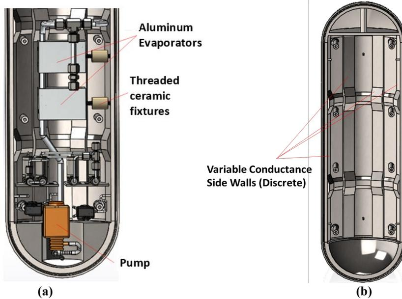
**Figure 3: (a) View of the P2P loop inside of one of the two shells of the melting probe prototype (b) Discrete and rectangular VCHP walls embedded within the shell walls of the melting probe prototype**
