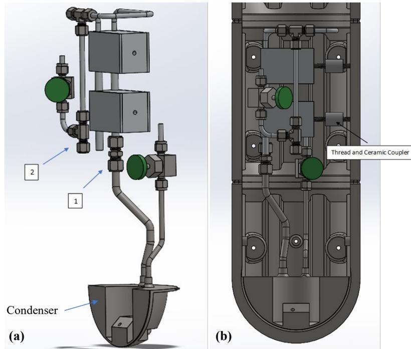
**Figure 10: (a) Condenser and evaporator assembly, (b) Condenser and evaporator assembly fit into probe shell**
