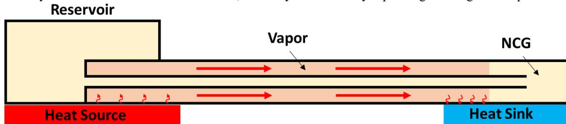
Figure 2. Hot-reservoir VCHP. NCG reservoir is closely integrated with the evaporator and follows the heat source temperature.
