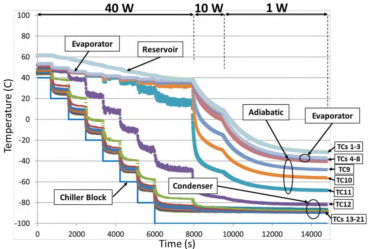
Figure 13. Thermal control test of the Astrobotic hot-reservoir hybrid-wick VCHP. Initial conditions: Power = 40W, Chiller Block Setpoint = 40°C, Evaporator Operating Temperature = 53.6°C. Refer to Figure 11 for TC numbers.
