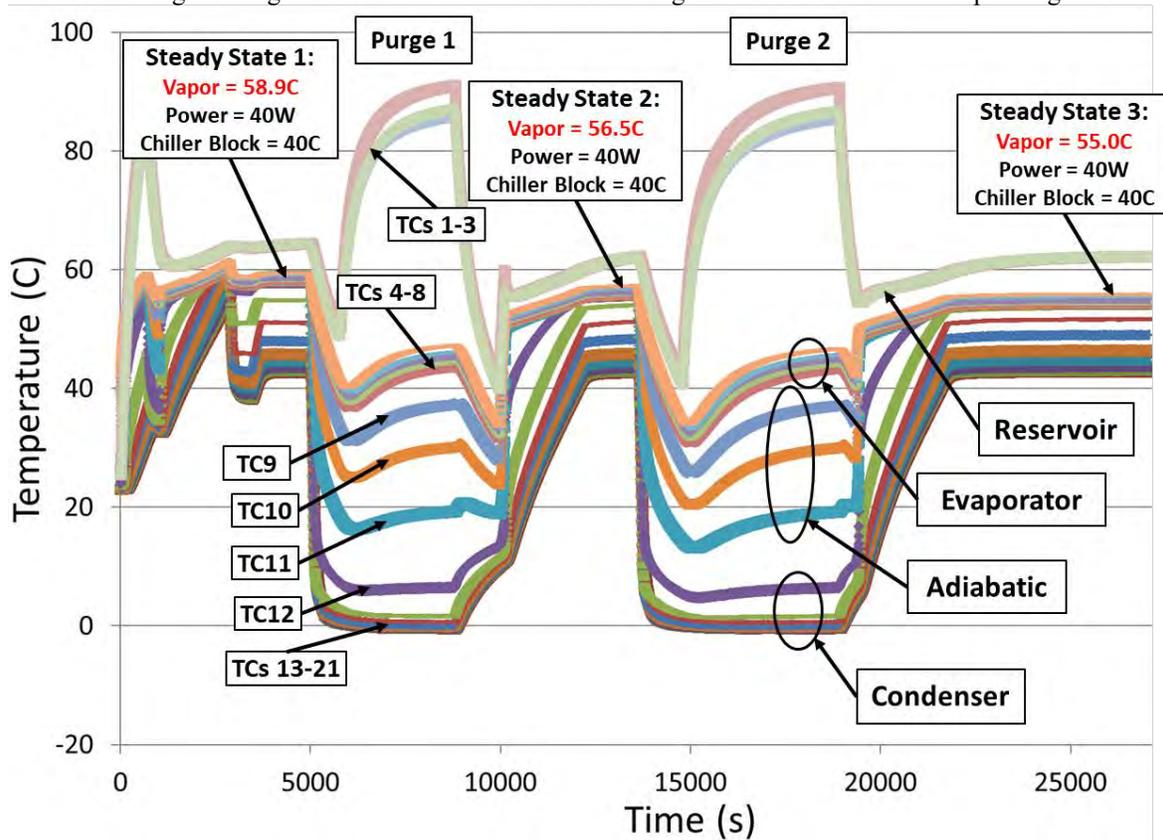
Figure 16. Example of two subsequent purge tests of the Astrobotic non-integrated hot-reservoir VCHP. Test was initiated after several days of non-operation allowing working fluid to diffuse into the NCG reservoir resulting in a higher steady-state operating temperature. During the Purge tests, power to the evaporator was turned off and 12W of heater power was applied directly to the NCG reservoir using a dedicated heater. Refer to Figure 11 for TC numbers.
