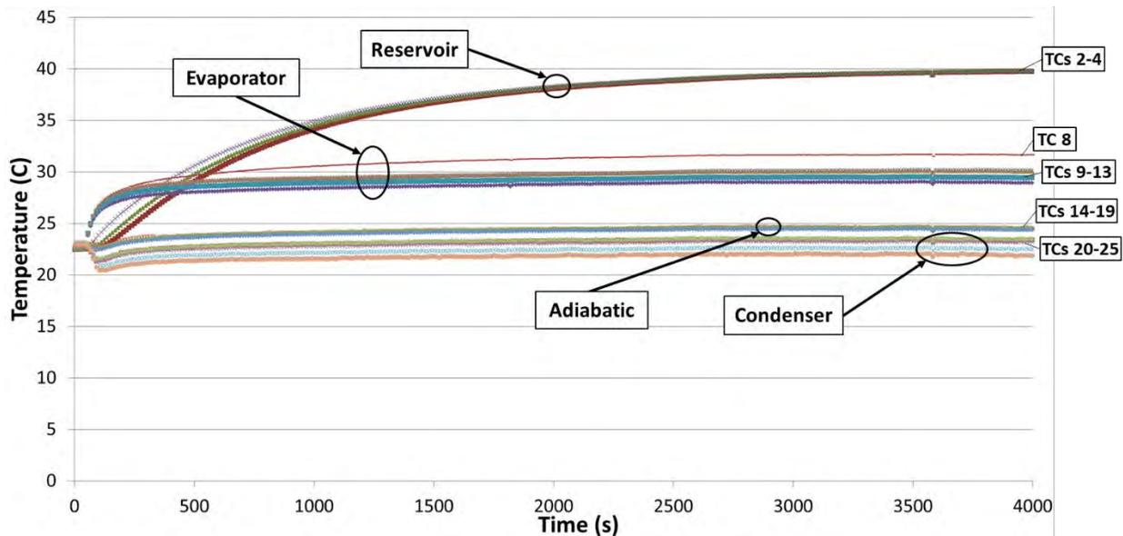
Figure 6. Temperature observed during different stages of the VIPER VCHP startup in a vertical orientation. Startup conditions included Power of  $147\text{W}$ . Chiller Block Setpoint at  $15^{\circ}\text{C}$ . Refer to Figure 4 for TC numbers.
