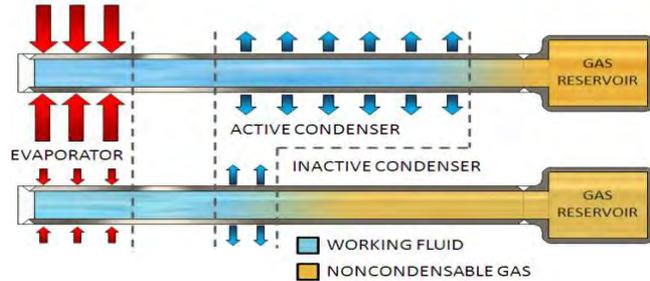
Figure 1. Operation of a cold-reservoir VCHP.
