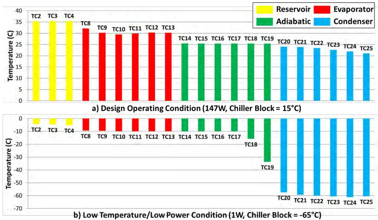
Figure 8. Comparison of instantaneous temperature distribution along the VIPER VCHP during a) the design operating condition and b) the low temperature/low power condition. Refer to Figure 4 for TC numbers.
