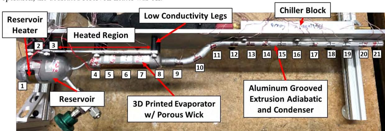
Figure 11. Image of the completed aluminum-ammonia non-integrated hot-reservoir hybrid wick VCHP for Astrobotic’s Lunar Lander Peregrine I. Locations of numbered TCs are indicated.
