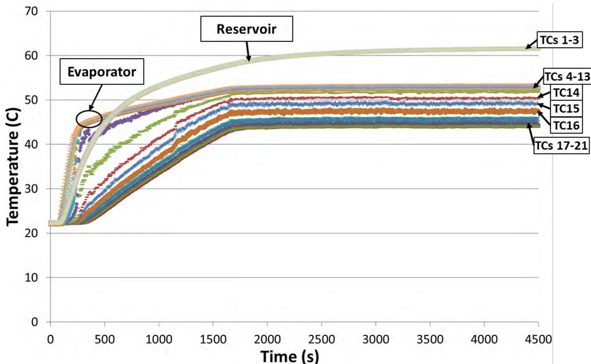
**Figure 12. Startup of Astrobotic hot-reservoir hybrid-wick VCHP in the vertical orientation. Power = 40W. Chiller Block Setpoint temperature = 40°C. Refer to Figure 11 for TC numbers.**
