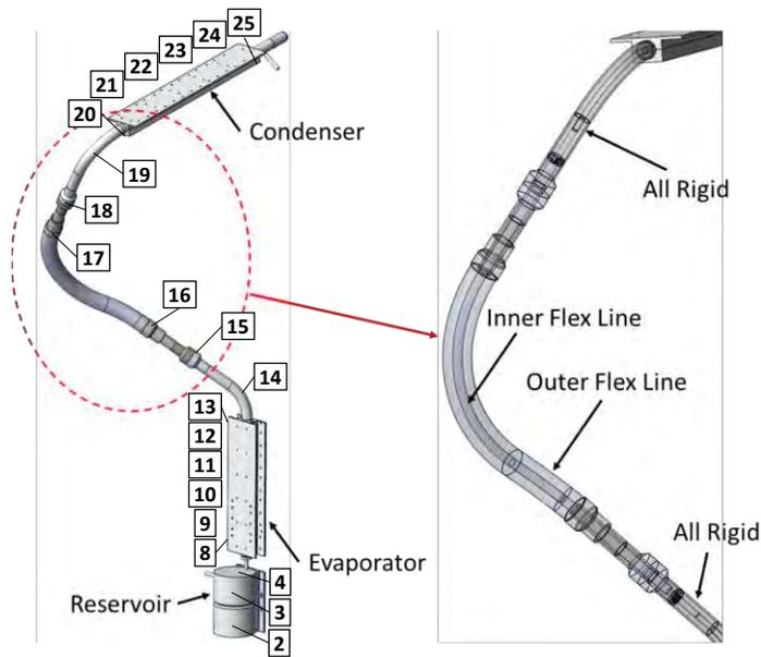
**Figure 4. Model of the VCHP designed and fabricated as part of NASA's VIPER Thermal Management System Engineering Demonstration Unit. Locations of numbered TCs are indicated.**
