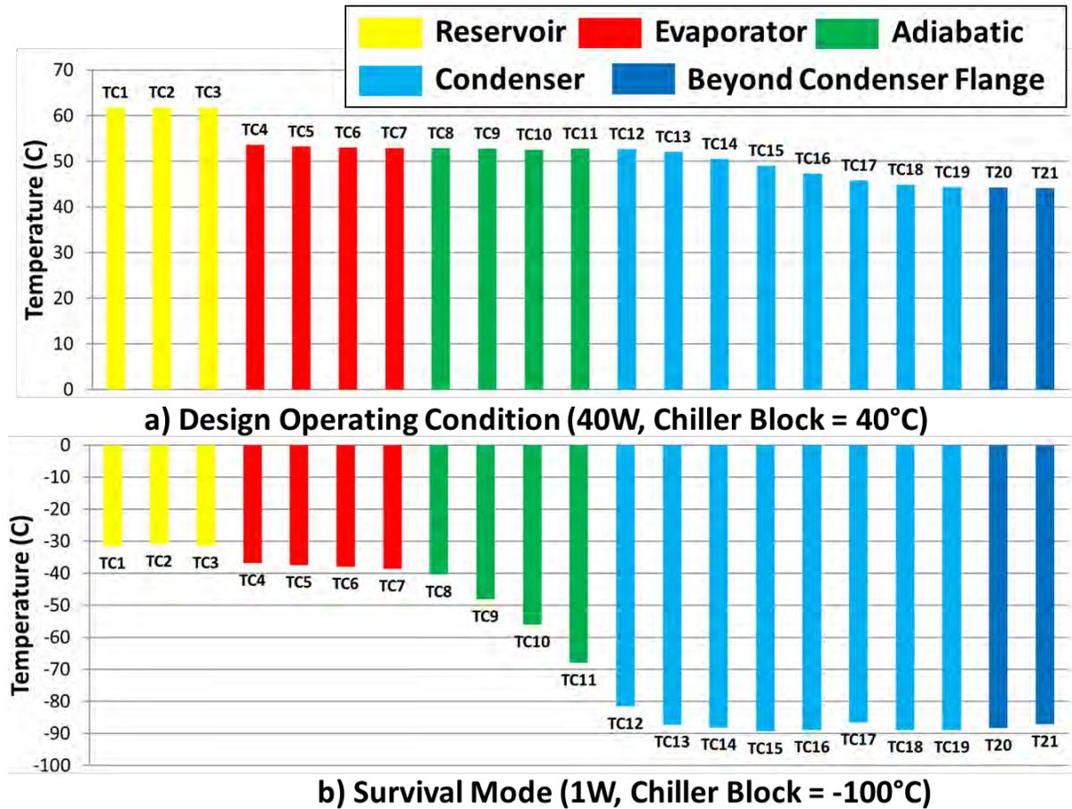
Figure 15. Comparison of instantaneous temperature distribution along the Astrobotic VCHP during a) the design operating condition and b) the low temperature/low power survival condition. Refer to Figure 11 for TC numbers.
