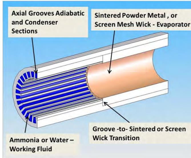
Figure 3. Hybrid wick for planetary surface and high heat flux applications.<sup>2</sup>
