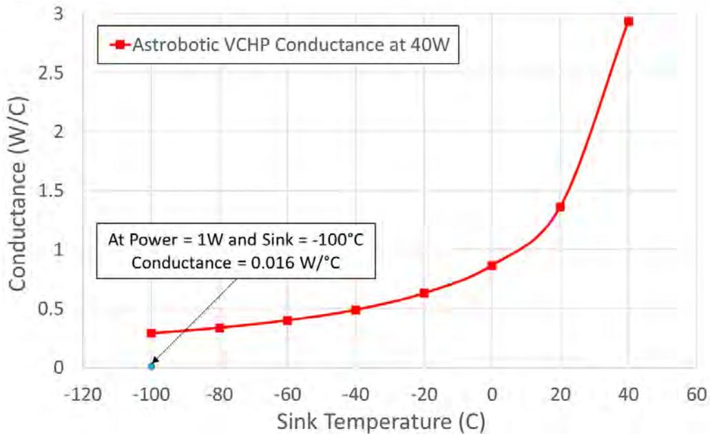
Figure 14. Variation in conductance of the Astrobotic VCHP with sink temperature at a fixed power of 40W. The conductance at the minimum sink temperature and 1W applied power is also indicated.
