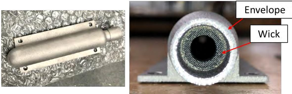
**Figure 9. Images of the 3D-printed aluminum evaporator for the Astrobotic VCHP. The porous wick and solid wall were simultaneously printed as one continuous part.**
