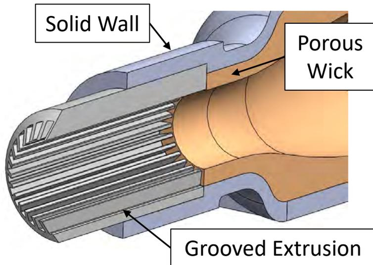
**Figure 10. CAD model of aluminum grooved extrusion interfacing with 3D-printed porous wick of the evaporator for the Astrobotic**
