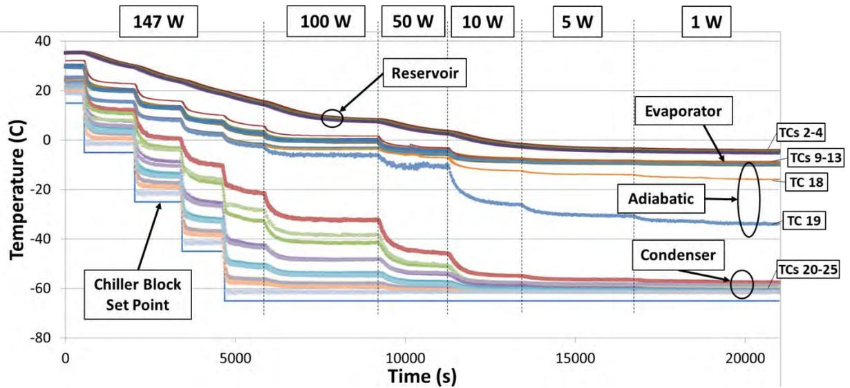
Figure 7. Thermal control test of VIPER VCHP. Minimum chiller block setpoint was  $-65^{\circ}\text{C}$  to avoid freezing of the working fluid. The initial phase of the test demonstrates reducing sink temperature at constant power. This was followed by reducing the power with constant sink temperature. Refer to Figure 4 for TC numbers.
