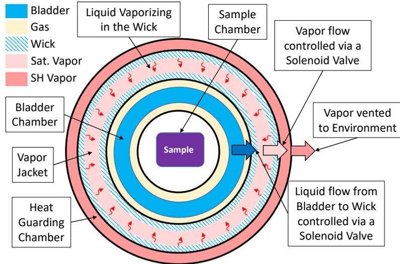
**Figure 1. Illustration of Vapor-Venting Thermal Management System. Working fluid within a Vapor Jacket absorbs heat through vaporization and vapor is vented from the system. The wick is supplied with liquid from a positive expulsion bladder.**
