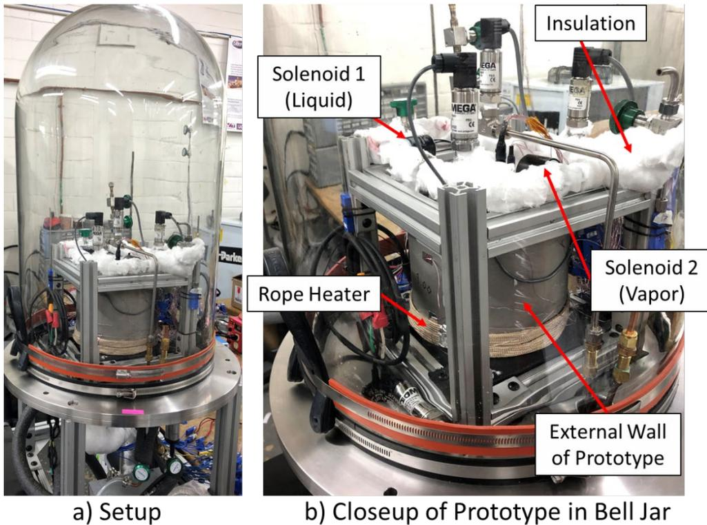
**Figure 7. a) Image of the entire experimental setup, b) closeup of the prototype in the bell jar. The external plumbing was covered with insulation. A rope heater was wrapped around the prototype.**
