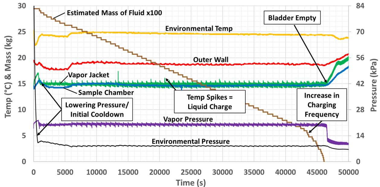
**Figure 8.** Time history of temperature measurements on the Phase I prototype during testing. The setpoint temperature was controlled by a TC on the wall separating the vapor jacket and bladder chamber, labelled “Vapor Jacket” in the plot. Temperatures and “Estimated Mass of Fluid×100” are read on the left axis and pressure is read on the right axis. Dividing “Estimated Mass of Fluid×100” by 100 gives the mass of fluid in kg. The initial mass of acetone was 0.294 kg.
