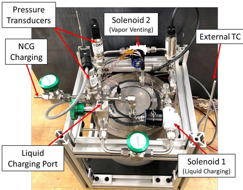
Figure 6. Image of the Phase I prototype. Various components for liquid distribution and control are labeled.
