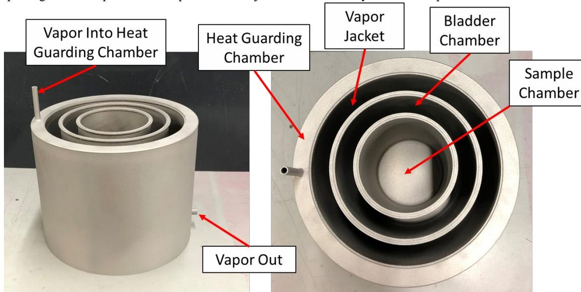
**Figure 4. Images of the stainless-steel additively manufactured envelope of the Phase I prototype. Annular end caps (not shown) were used to close the vapor and bladder chambers. A circular disk end cap (not shown) was used to close the sample chamber.**
