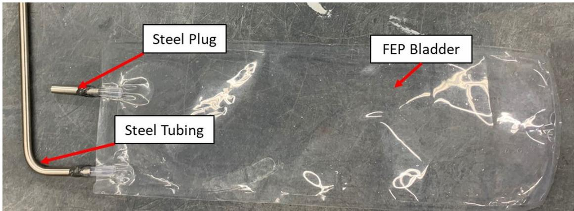
Figure 5. Image of FEP bladder used in Phase I Prototype. The bag was manufactured with two ports. One port was plugged with a stainless-steel rod. A stainless-steel tube was connected to the other port for charging and discharging the bladder.
