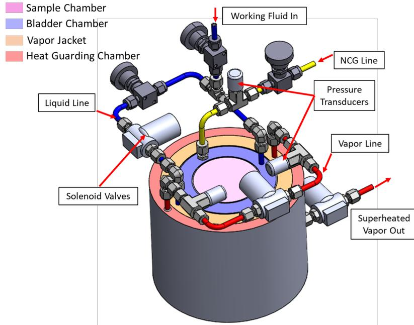
**Figure 2. 3D model of the Phase I prototype showing the valve and plumbing system for fluid distribution and control.**
