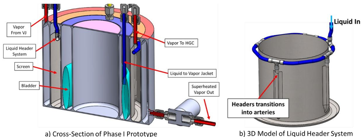
**Figure 3. a) Cross-section showing the internal structure of the Phase I VVTMS Prototype design. b) 3D model of the liquid header system that fed liquid into the screen within the vapor jacket.**
