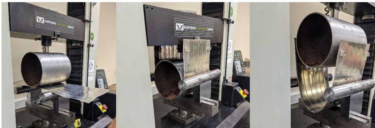
Figure 7. Sequence of images showing the initial bending step performed by EWI. Left – Panel loaded into test frame. Center – Panel Bend to 90°. Right – Center die removed from panel.
