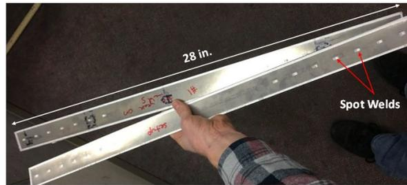
a) Single-channel prototypes prior to heat treatment
