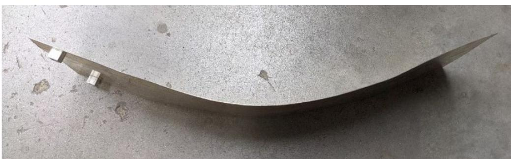
Figure 8. Panel after being removed from the bending fixture. After removing the panel from the bending fixture significant spring back was observed.
