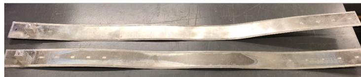
b) Single-channel prototypes after heat treatment
