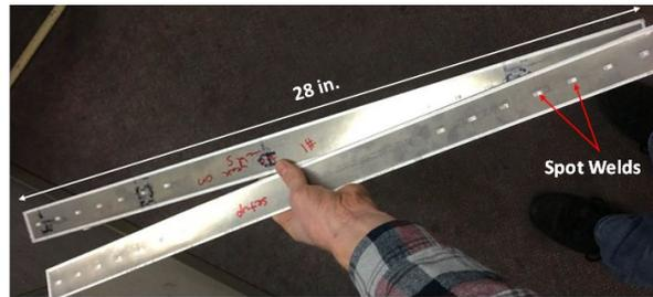
a) Single-channel prototypes prior to heat treatment
