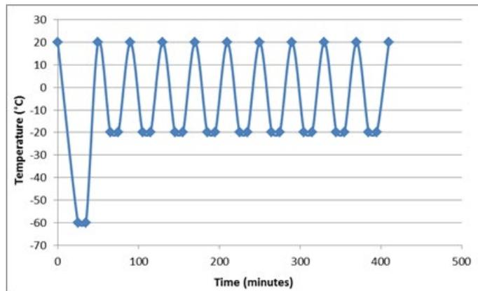
Figure 13. Freeze/Thaw cycle data for the Liquid Wicked Reservoir.
