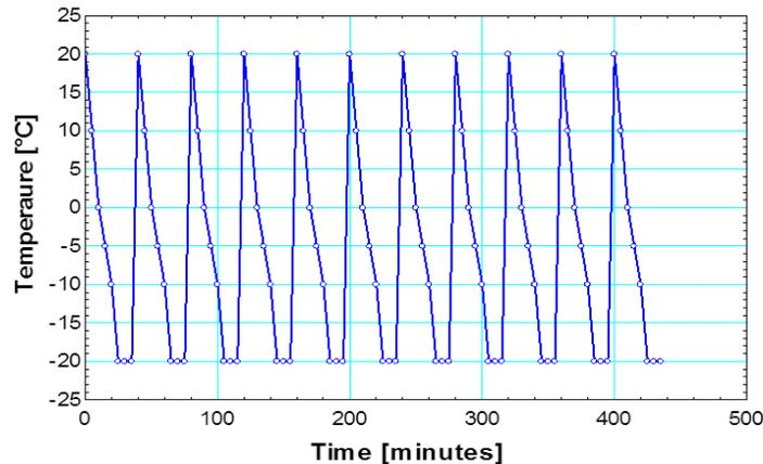
**Figure 10. Freeze/Thaw cycle data for the internal buffer prototype.**
