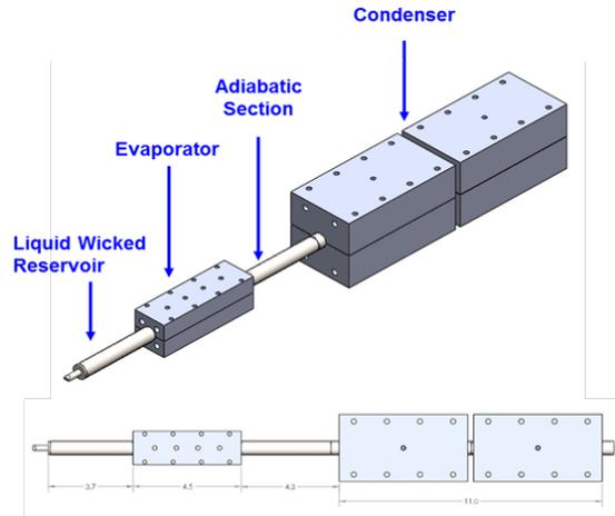
Figure 14. Test setup for the un-flanged titanium/water heat pipe.
