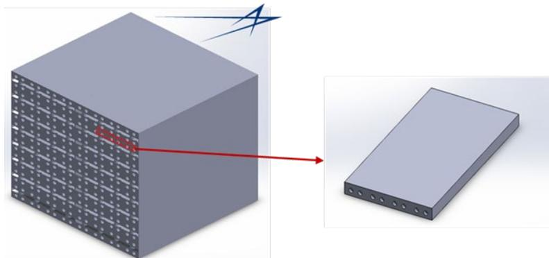
Figure 19. The Dragonfly high-power T/R module (Left), single quad pack unit with 8 SSPAs (Right).
