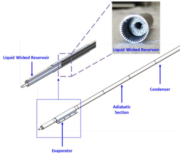
Figure 12. 3D Printed grooved heat pipe with the Liquid Wicked Reservoir in the evaporator section for freeze protection.
