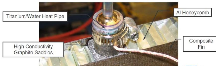
**Figure 1. Initial titanium heat pipe/POCO Foam Saddle/GFRC radiator design (Anderson et al., 2006a)**
