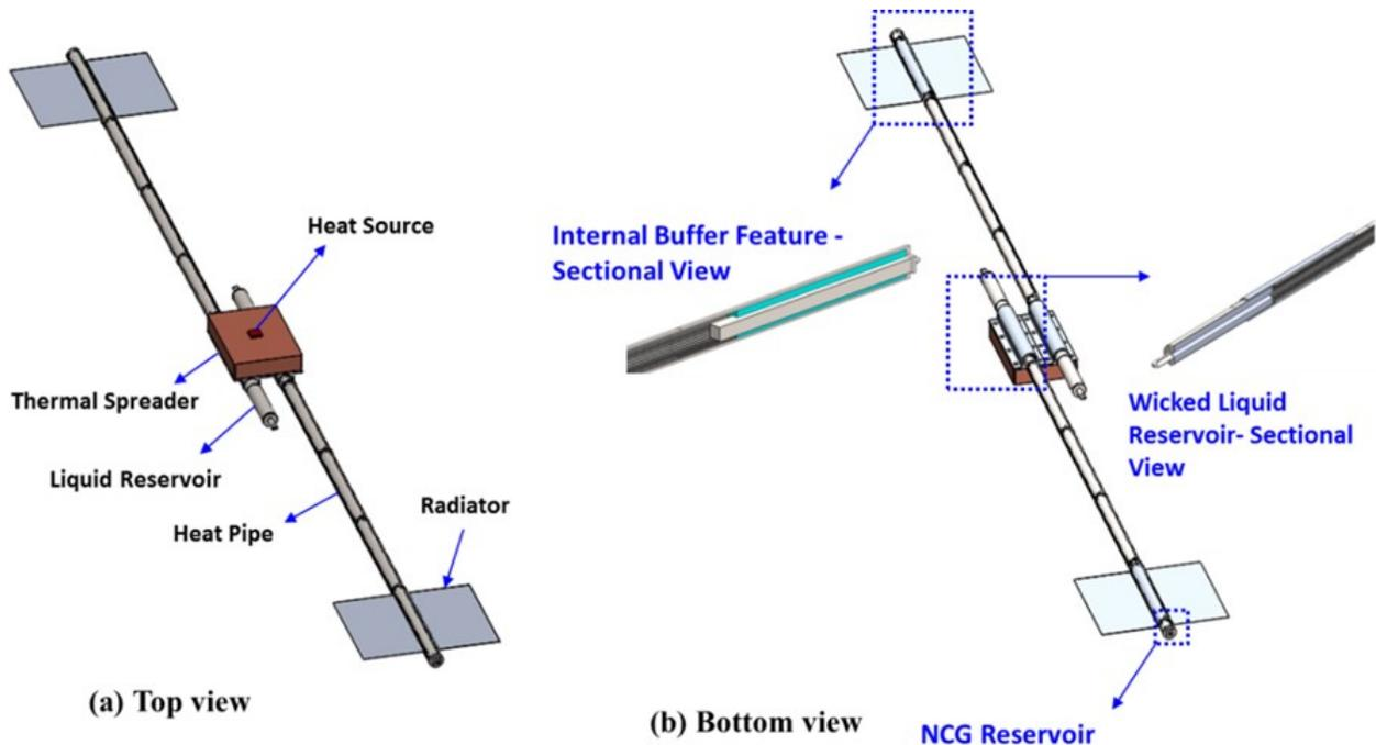
**Figure 3. Thermal Management System Schematic for Future GaN SSPA Devices (a) Top view. (b) Bottom view.**
