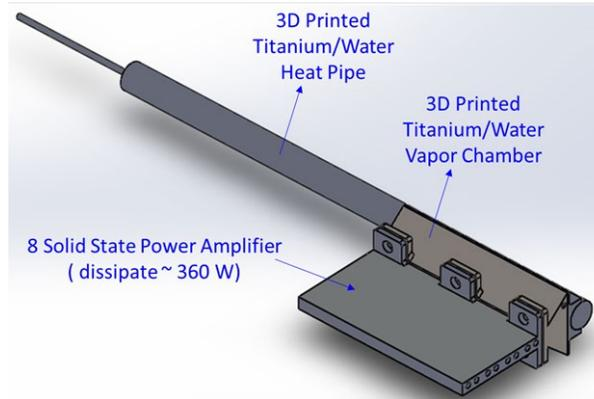
**Figure 20. Thermal management design for the subscale (i.e. quad pack) Dragonfly high-power T/R module.**
