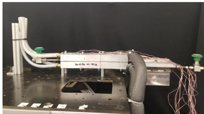
**Figure 25. Thermal management system under testing for the subscale (i.e. quad pack) Dragonfly high-power T/R module.**
