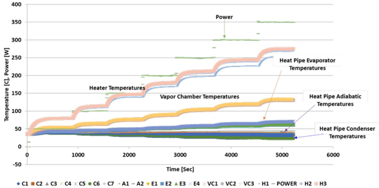
Figure 26. Thermal performance for the 3D printed thermal management system for the subscale (i.e. quad pack) Dragonfly high-power T/R module with s-bond as TIM.
