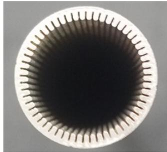
**Figure 21. Cross sectional view of the 3D printed titanium heat pipe with 57 grooves.**
