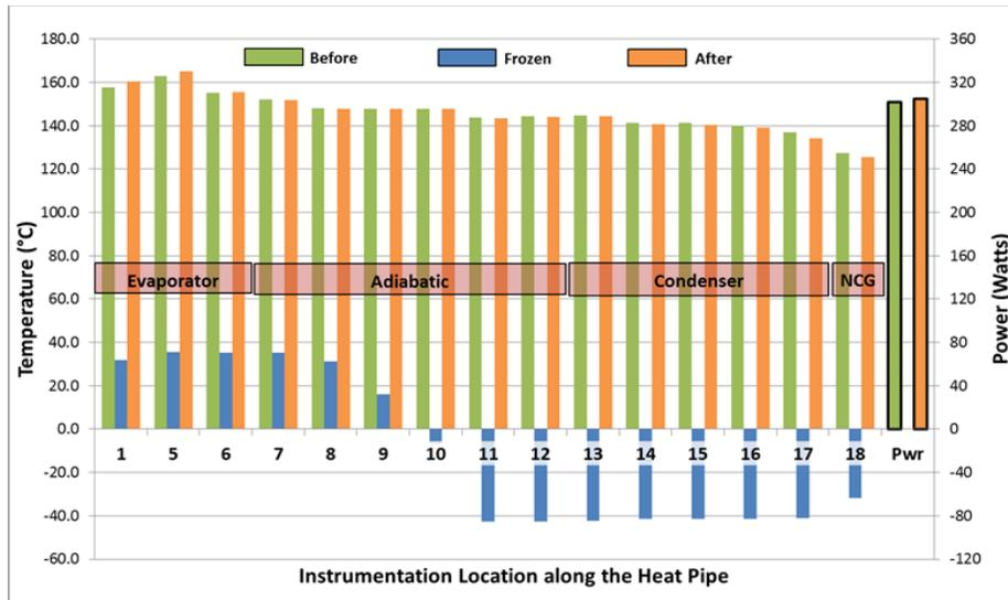
Figure 18. Grooved heat pipe instantaneous temperature profiles before, during, and after start-up from a frozen state.
