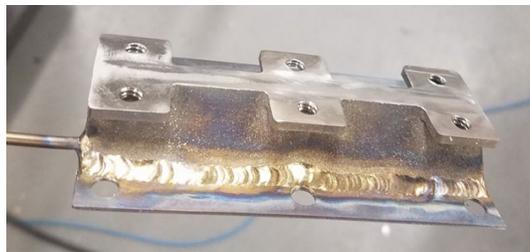
**Figure 23. Titanium vapor chamber for SSPA cooling, with bolts to connect to the simulated GaN amplifier plate.**
