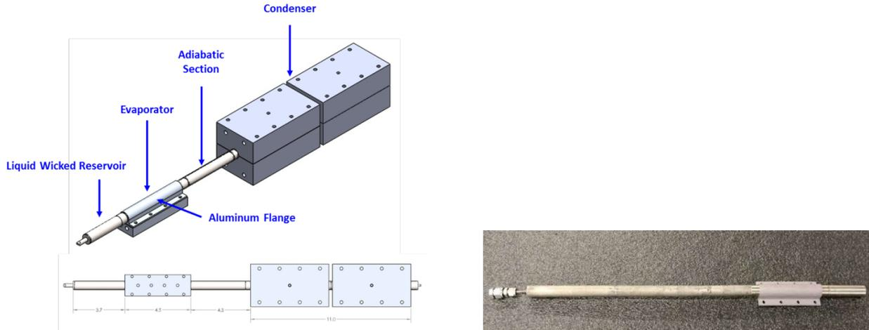
**Figure 16. The flanged titanium/water heat pipe.**
