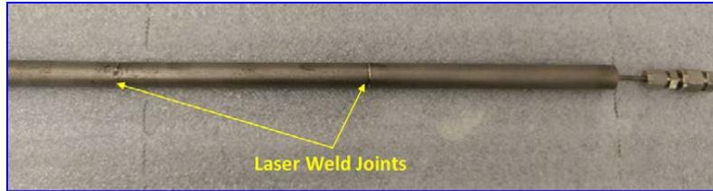
**Figure 6. Laser-Beam Welding was used to join the 3D printed grooved sections.**
