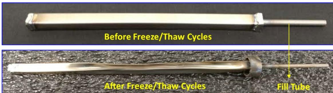
**Figure 11. The full-scale internal buffer before and after 10 Freeze/Thaw cycles.**
