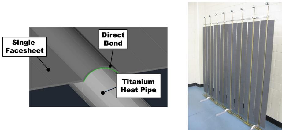
**Figure 2. a. Direct bond concept. b. Single face-sheet titanium heat pipe radiator direct bonded to GFRC facesheets. (Tarau et al., 2016)**
