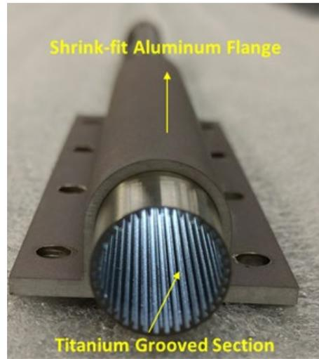
**Figure 7. The aluminum flange was joined to the titanium heat pipe via shrink-fit.**
