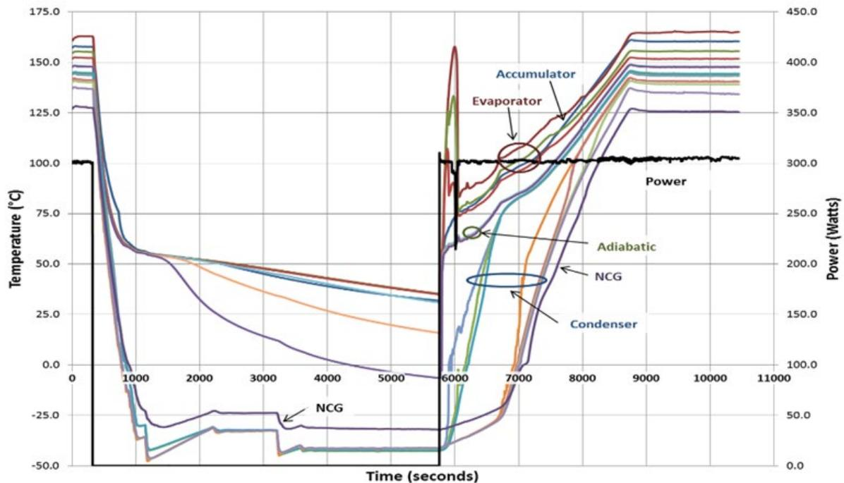
**Figure 17. Grooved heat pipe start-up transient temperature profile from a frozen state.**
