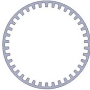
**Figure 4.** The grooves in the selected heat pipe geometry are square, allowing water to expand into the vapor space. Inverted trapezoidal wicks, wider at the I.D., have also been used successfully in the past.
