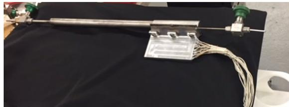
**Figure 24. Thermal management system, with the vapor chamber attached to the titanium-water heat pipe and to the heater block.**
