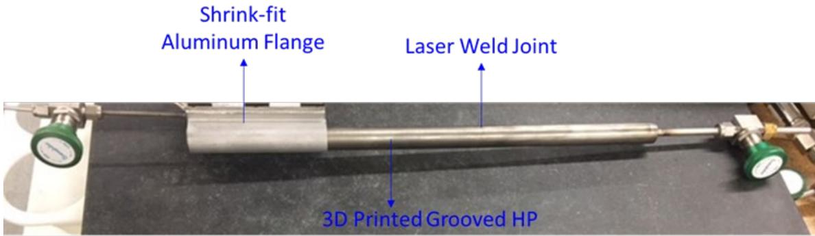
**Figure 22. Heat pipe for SSPA cooling with a shrink-fit aluminum flange.**
