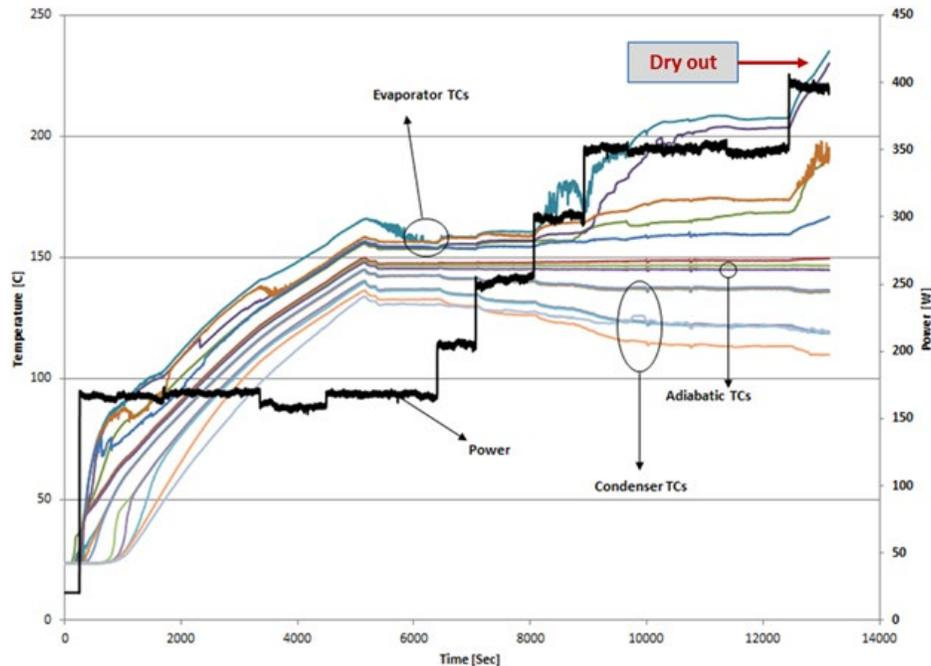
Figure 15. Thermal performance for the un-flanged 3D Printed grooved titanium-water heat pipe.
