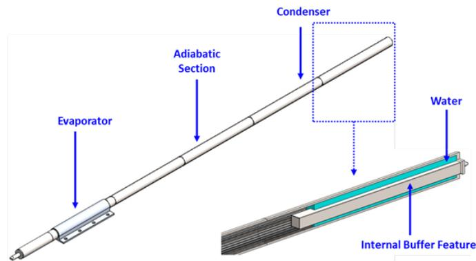
**Figure 8. CAD model of grooved heat pipe with internal buffer for freeze/thaw control in the condenser section.**
