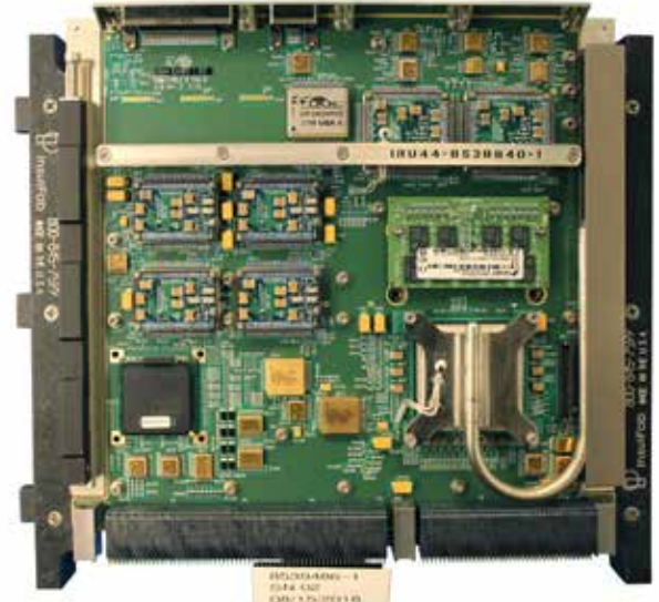
Figure 1: Photo courtesy of BAE systems, showing ACT SCWHP embedded in a BAE RAD5545™ Space VPX board
