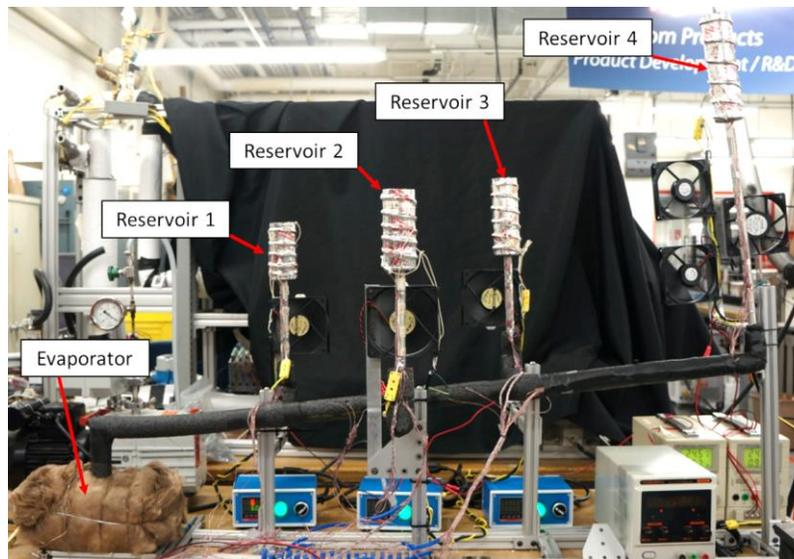
Figure 7. MCVCHP experimental prototype.
