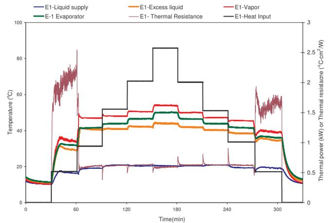
Figure 8 Temperature and thermal resistance variations of Evaporator #1.
