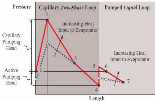
**Figure 2 Pressure profile of hybrid two-phase loop.**
