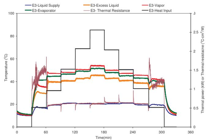
Figure 9 Temperature and thermal resistance variations of Evaporator #3.
