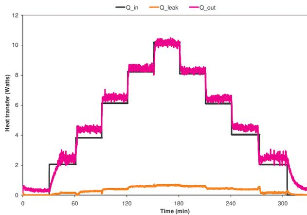
**Figure 11 Calorimetry of four-evaporator hybrid two-phase loop.**
