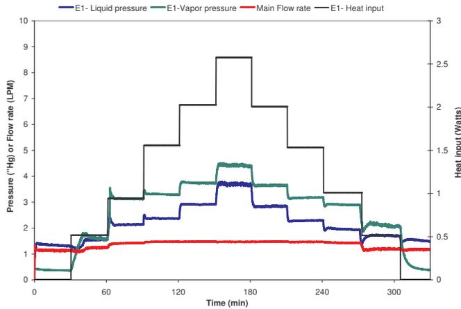
**Figure 10 Pressure and flow rate variations in Evaporator #1.**
