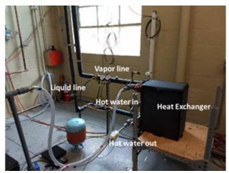
Figure 4. A flat plate heat exchanger connected to the loop thermosyphon and a recirculation water heater.
