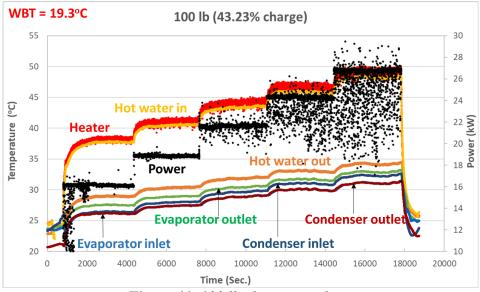
Figure 11. 100 lb charge test data.
