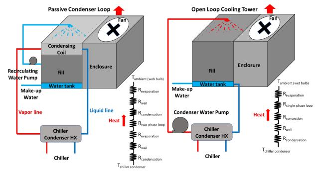
Figure 1. Schematics of the passive condenser loop and the open loop cooling tower. Note in the passive condenser loop, a small recirculating pump is still needed for spraying the cooling water to the condensing coil, but the electrical energy consumption is much smaller compared to the condenser water pump in the open loop cooling tower.
