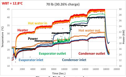
Figure 8. 70 lb charge test data.
