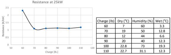
Figure 14. Left: Overall thermal resistance vs. fluid charge. Right: Wet bulb temperature at different charge tests.
