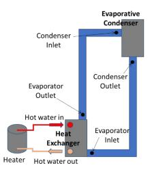
Figure 2. Schematic of the passive condenser loop test setup.
