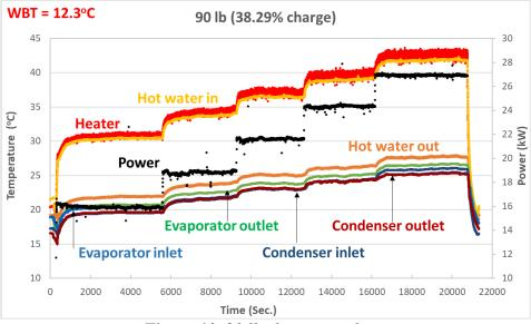
Figure 10. 90 lb charge test data.
