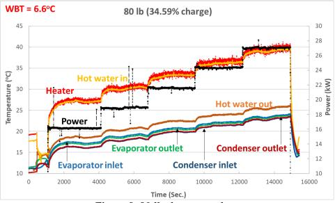
Figure 9. 80 lb charge test data.
