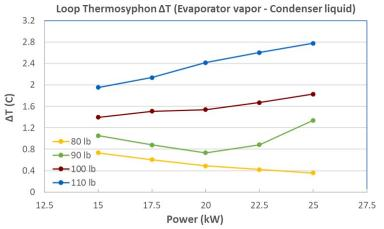
Figure 13. Loop thermosyphon  $\Delta T$  vs. input power for different fluid charges.
