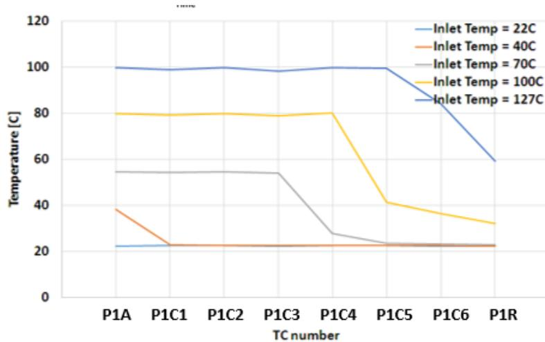
Figure 6. Steady state temperature profiles along Pipe No 1 corresponding to each water inlet temperature
