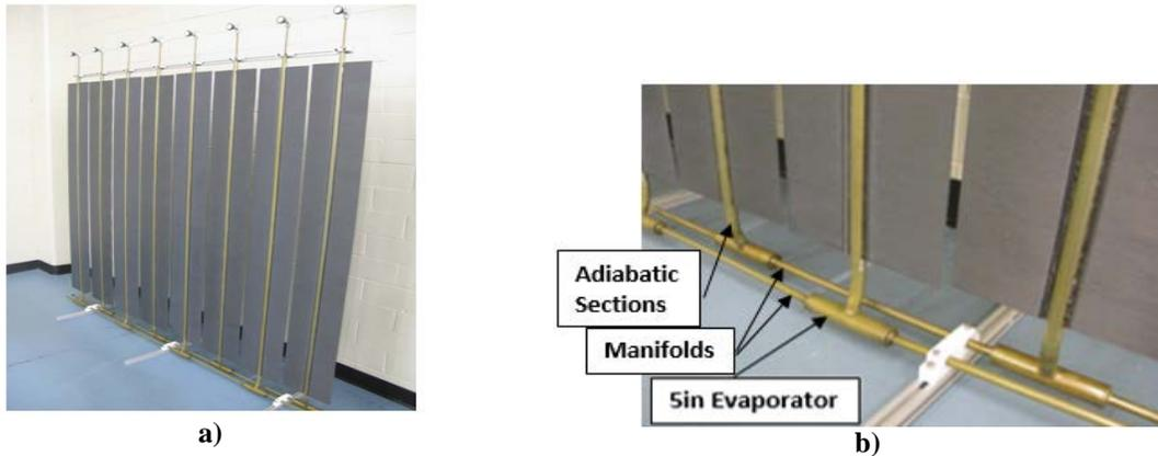
**Figure 3. First cluster a) Actual radiator cluster b) Detail showing the manifolds, the heat pipe evaporators and adiabatic sections**
