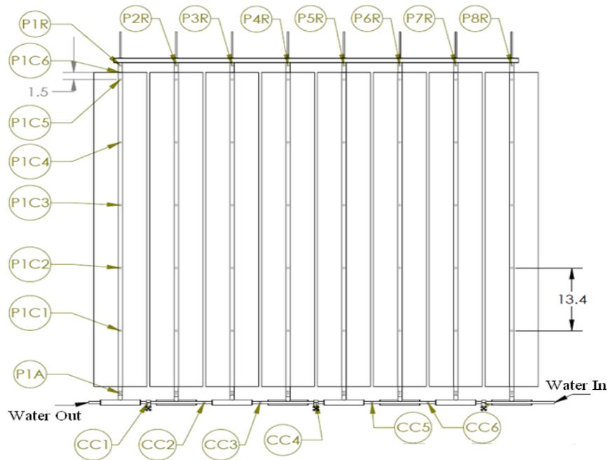
**Figure 4. Thermocouple map on the first cluster**
