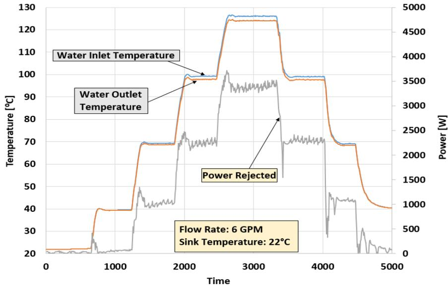
Figure 5. Power test: heat rejected for various water inlet temperatures
