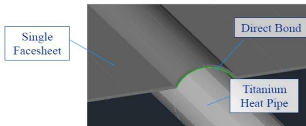
Figure 2. Single facesheet radiator with direct bonding of the facesheet to the heat pipes<sup>4</sup>
