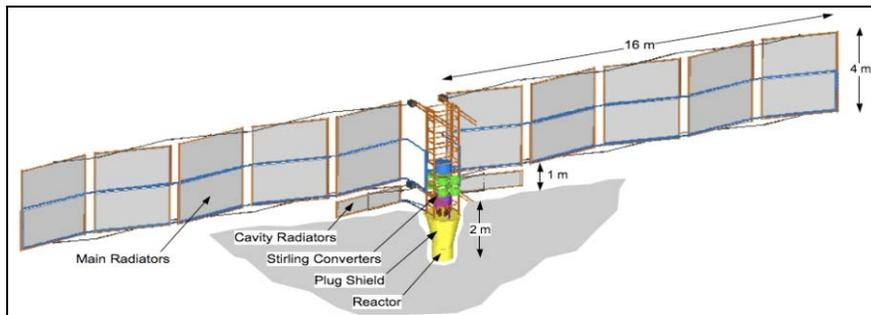
Figure 1. Fission surface power system concept<sup>2</sup>
