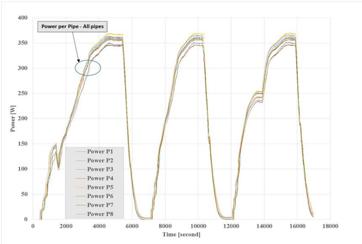
Figure 10. Power dissipated by each individual module/condenser
