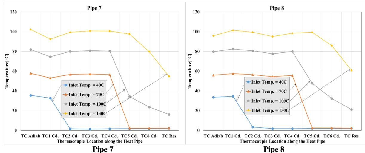
**Figure 11. Steady state temperature profiles along each of the eight heat pipes during the second round of vacuum testing at GRC when maximum outlet water temperature was 127°C**
