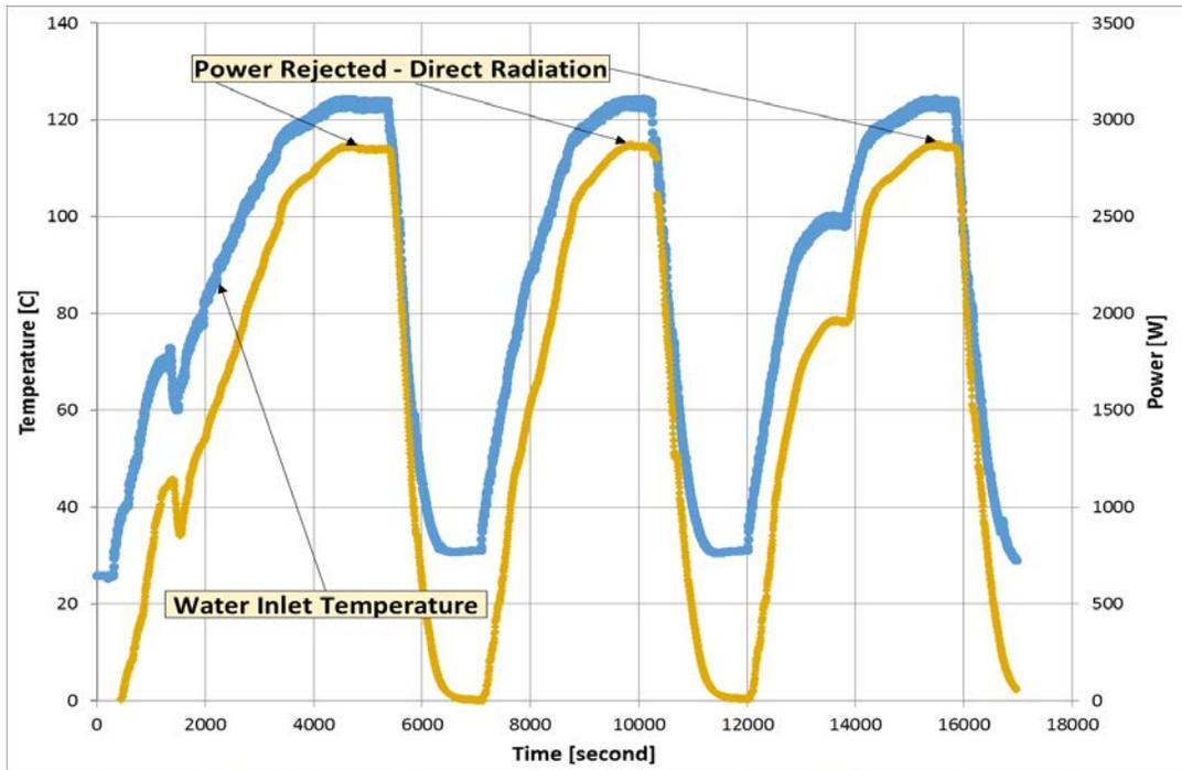
Figure 9. Power rejected in vacuum during the second round of testing when maximum inlet water temperature was 127°C
