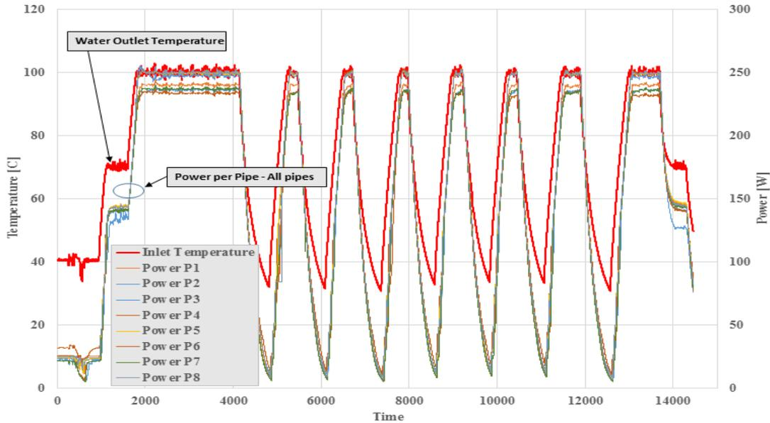
**Figure 8. Power rejected by each module to validate the calculation method that was used to evaluate the total power during the first round of vacuum testing (max outlet water temperature was 100°C)**
