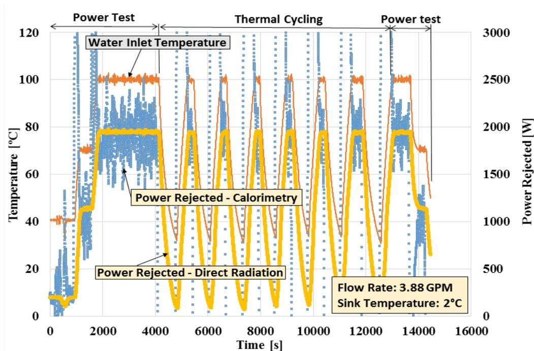
**Figure 7. Radiator cluster testing in vacuum – first round. Testing was carried as power test, thermocycling and power test again.**
