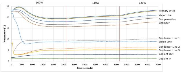
Figure 10. Steady state testing of LHP after vibration testing with flexible lines
