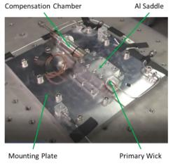
Figure 9. LHP evaporator assembly on vibration table for testing
