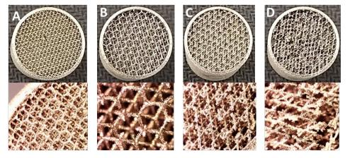
Figure 11. 3D printed secondary wicks using a defined lattice structure.
