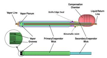
Figure 2. Detailed view of LHP evaporator
