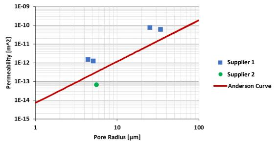
Figure 13. Pore size and permeability testing result of new wick samples demonstrating higher permeabilities than previous wicks
