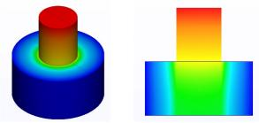
Figure 16. Temperature contour calculated based on Fourier's diffusion law, which can be analogized to the pressure in the Darcy's law.
