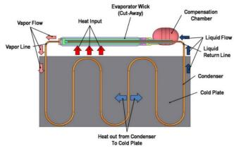
Figure 1. Loop heat pipe schematic (not to scale).
