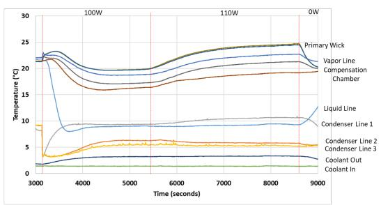
Figure 6. Steady state testing of prototype at an adverse elevation of 5.25" with both the evaporator and condenser flat
