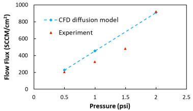
Figure 17. A comparison between experimental measurement and CFD diffusion model of the 3D printed bipore size sample.
