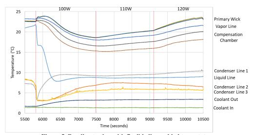
Figure 5. Baseline testing with flexible lines added to prototype
