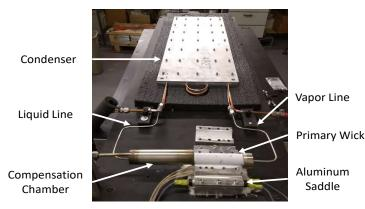
Figure 4. Completed LHP prototype with 3D printed primary wick
