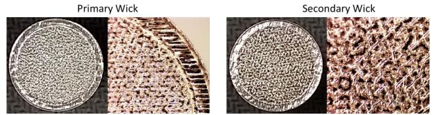
Figure 12. Images of 3D printed wick samples from a second supplier.
