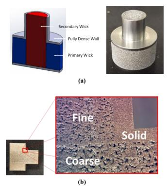
Figure 14. (a) Test sample with combined primary and secondary wicks. (b) Section through a primary/secondary wick sample, showing the interfaces between the two wicks, and between the wicks and solid envelope.
