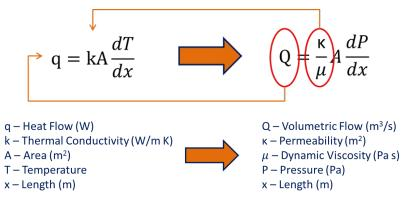
Figure 15. The corresponding terms of thermal (Fourier's Law) and fluid (Darcy's Law) analogy.
