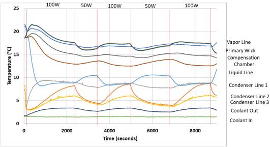
Figure 8. Power cycle testing of prototype with evaporator tilted at 25° against gravity
