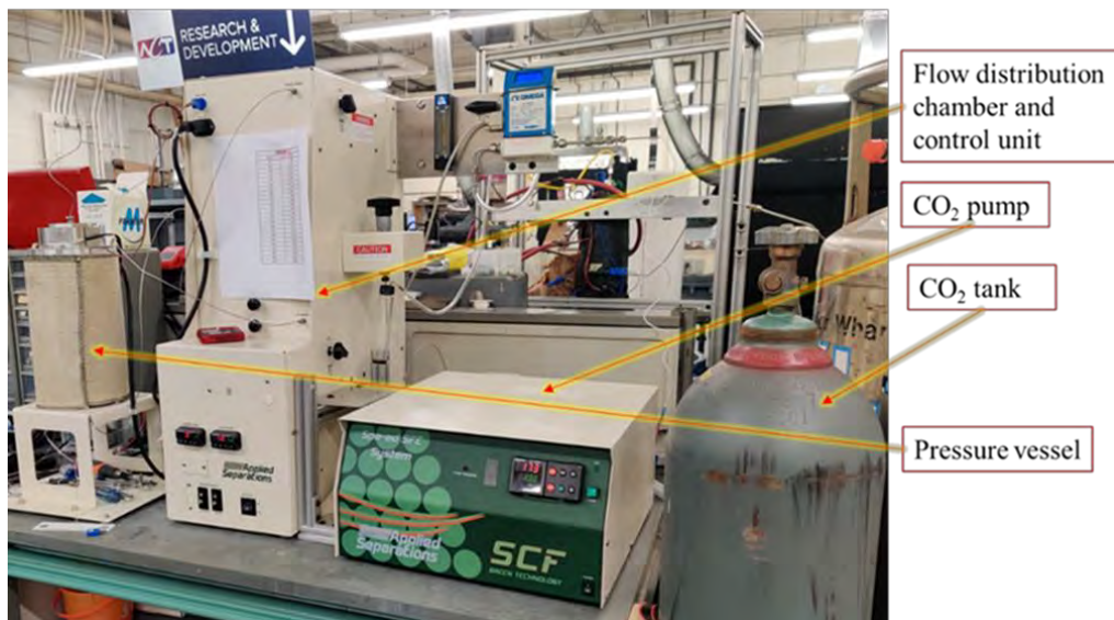
Figure 2. Supercritical fluid (CO 2 ) extraction system [15]
