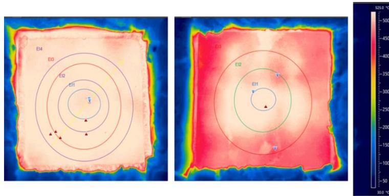
Figure 9. (Left) IR image of the vapor chamber surface at 500 °C and (Right) IR image of an Inconel 600 block with embedded heaters at 500 °C.
