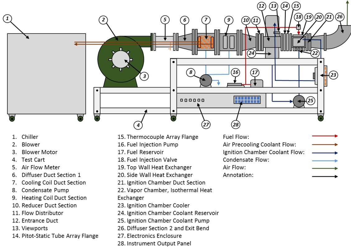
**Figure 3. Schematic of the HSI test apparatus design outlining the major components.**
