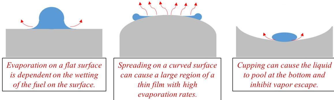
**Figure 7. Evaporation of a fuel droplet on flat, curved, and cupped hot surface.**
