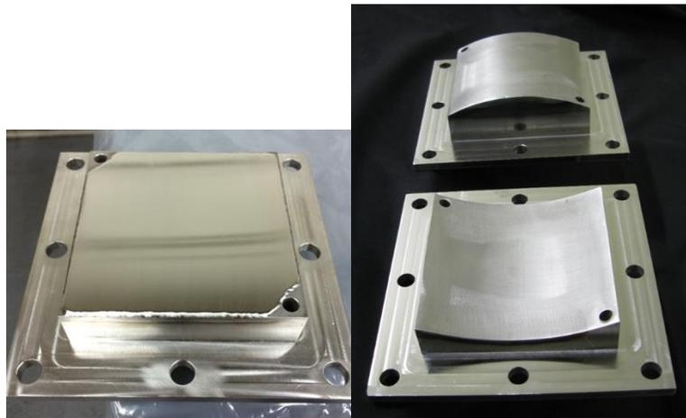
**Figure 8. Flat, convex, and concave vapor chambers for HSI testing.**
