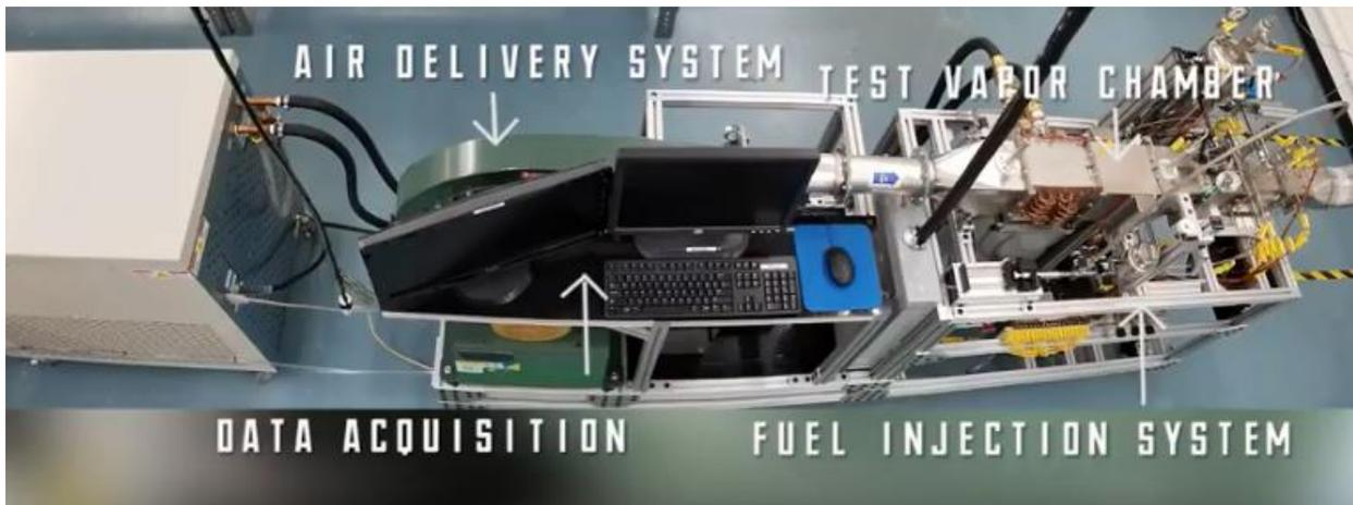
**Figure 4. Hot surface ignition test apparatus developed at ACT.**
