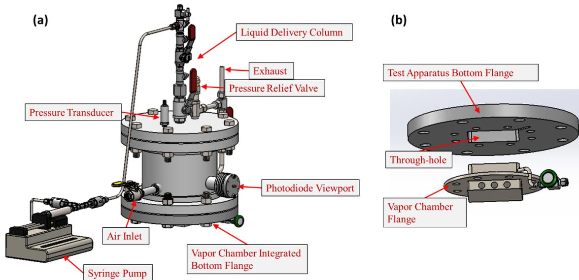
Figure 2. Prototype Design of vapor chamber based HSI testing chamber: (a) Overall apparatus used for testing, (b) Vapor chamber integrated into the bottom flange.
