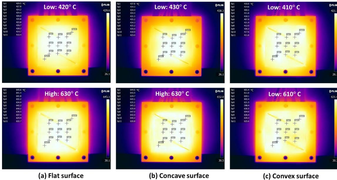
Figure 10. Thermal imaging of the hot surface vapor chambers, demonstrating isothermal operation.
