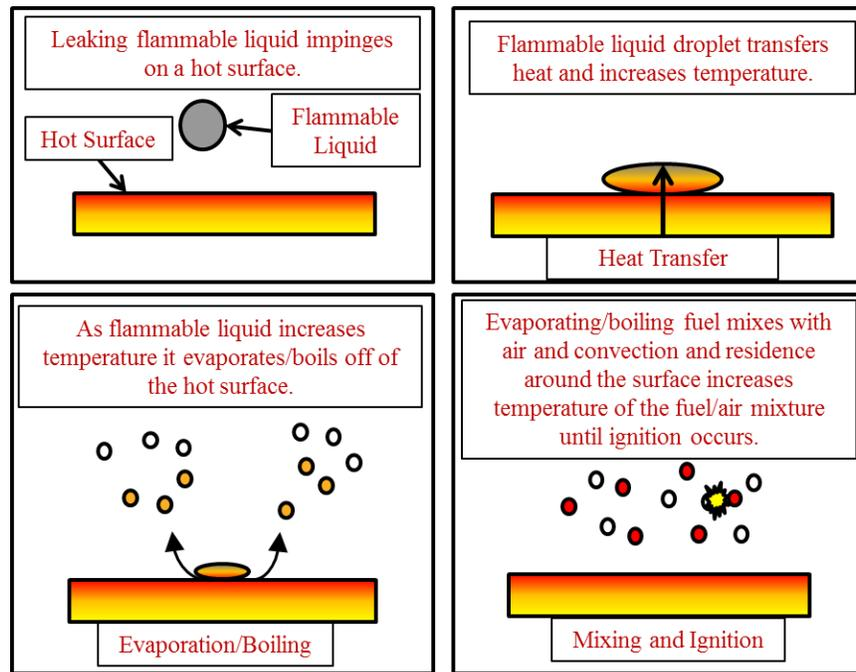
Figure 1. Illustration of the hot surface ignition process outlining the steps leading to ignition.
