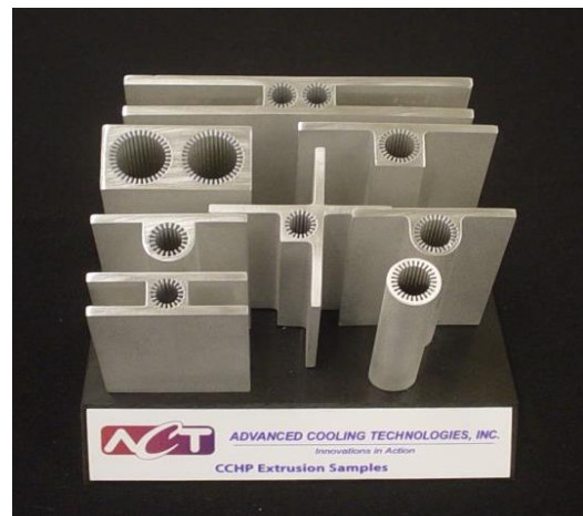
Fig. 2. Grooved aluminum extrusions for ammonia heat pipes. Grooves allow heat transfer over long distances for spacecraft applications, but only work about 0.10 inch against gravity for earth-based testing.
