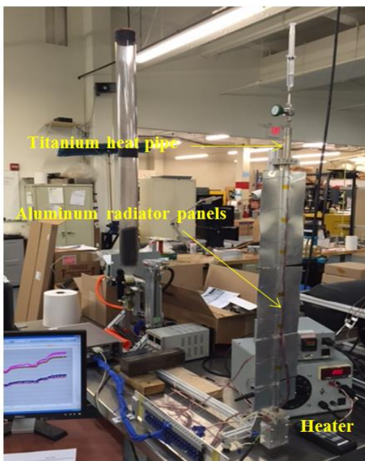
Fig. 10. Testing the titanium/aluminum radiator system in ambient conditions.
