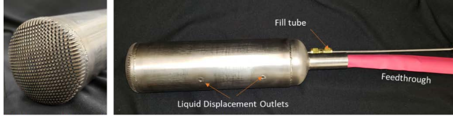
Figure 8. Lab-scale ice melting probe prototype with area enhanced melting head
