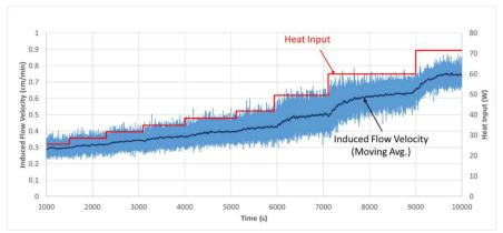
Figure 14. Momentum transport induced flow rate increases as the heat input increases
