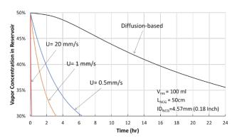
Figure 17. Convection-based purging rate vs. diffusion-based purging rate
