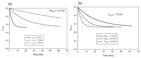
Figure 5. Variation of vapor concentration within reservoir with time for (a) various length of NCG tubes (ID 1.2 mm) and (b) various NCG tube diameters
