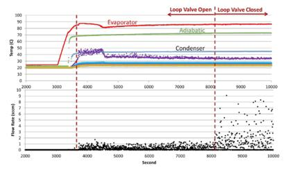
Figure 13. Temperature of VCHP Loop vs. secondary flow rate
