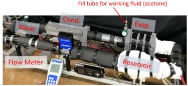
Figure 11. Experimental apparatus of the VCHP loop concept demonstration
