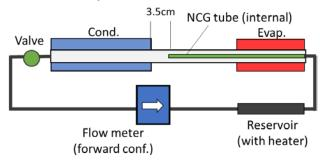
Figure 10. Schematic of experimental apparatus for Loop VCHP concept feasibility demonstration
