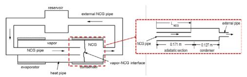
Figure 6. Schematic of VCHP loop
