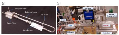
Figure 15. (a) Hot Reserovir VCHP Loop prototype (b) testing system
