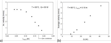
Figure 7. (a) Average velocity through NCG pipe vs. NCG pipe outlet location. (b) Average velocity through NCG pipe vs. heat input
