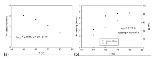
Figure 8. (a) Induced flow velocity vs. temperature with constant Q (b) Induced flow velocity and Q vs. temperature with constant heat transfer coefficient for cooling
