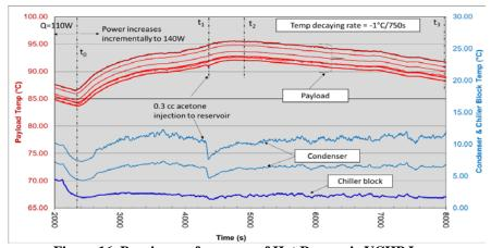
Figure 16. Purging performance of Hot Reserovir VCHP Loop
