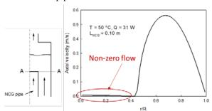
Figure 9. Velocity distribution across A-A section (induced flow velocity in the center is around 3 mm/s)
