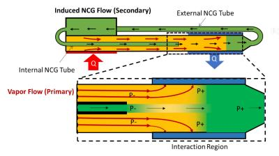
Figure 3. Loop Hot Reservoir VCHP (Green: NCG rich gas; Yellow: Vapor rich gas)
