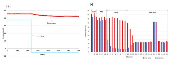
Figure 12. (a) VCHP test loop operation at 80 W with step change in sink temperature (b) Instantaneous heat pipe temperatures of VCHP test loop at 75  $^{\circ}$ C hot sink temperature and -10  $^{\circ}$ C cold sink temperature
