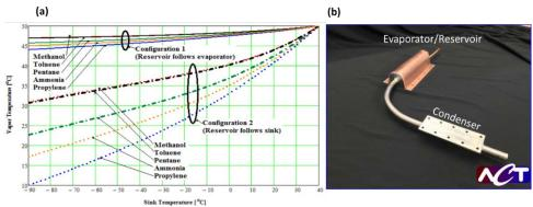
Figure 1. (a) Analytical thermal control predictions for two VCHP hot and cold reservoir configuration with five different working fluids: Methanol, Toluene, Pentane, Ammonia and Propylene<sup>3</sup> (b) VCHP with an integrated hot reservoir for ISS test
