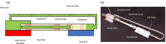
Figure 1. Advanced hot reservoir VCHP with (a) conceptual design of VCHP (b) proof-of-concept prototype developed in Phase I.
