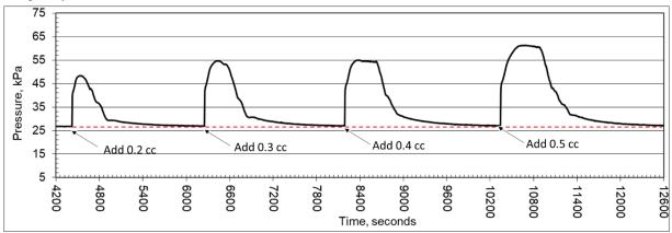
Figure 8. Repeatability test of VCHP loop purging (2-hole outlet).
