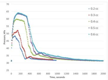
Figure 12. Purging rate with different added fluid volume into a warm reservoir.
