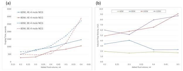
Figure 13. (a) Measured purging time with different heating powers and NCG amount (b) estimated bulk momentum-induced flow velocity under different heating powers with NCG of  $4x10^{-4}$  moles.
