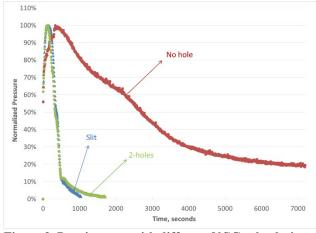
Figure 9. Purging rate with different NCG tube designs.
