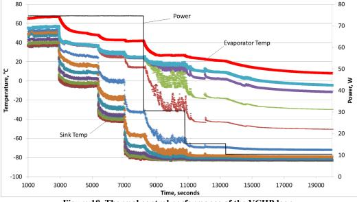
Figure 18. Thermal control performance of the VCHP loop.
