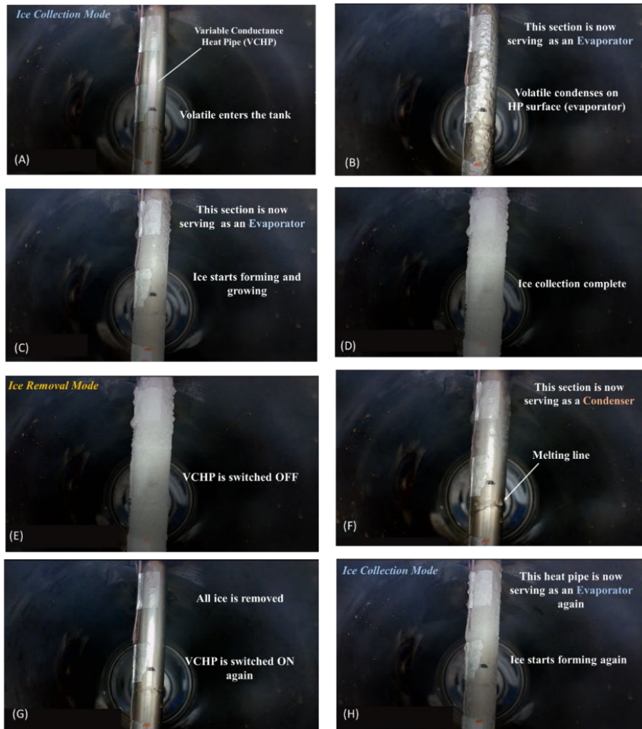
Figure 15. Demonstration of VCHP cold trap concept (A) volatile enters the tank (B) volatile start condensing and freezing on the heat pipe surfaces, that are serving as evaporators (C) ice layer becomes thicker and thicker (D) the system needs to switch to ice removal mode (E) VCHP is switched OFF by heating the NCG reservoir (F) ice started being removed from the heat pipe sections, operating as a condenser (G) all ice has been removed and VCHP is switched back ON for next round of collection (H) ice starts forming again
