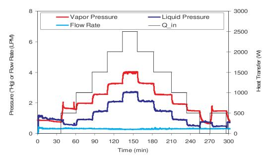
Figure 5 Pressure and liquid flow rate variation of hybrid cooling loop vs. heat input.
