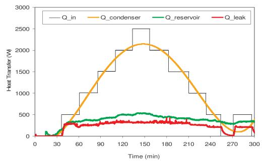
Figure 6 Calorimetery of hybrid cooling loop.
