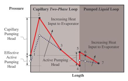
Figure 2 Pressure profile of hybrid cooling loop as the heat input to evaporator increases at constant pump speed.
