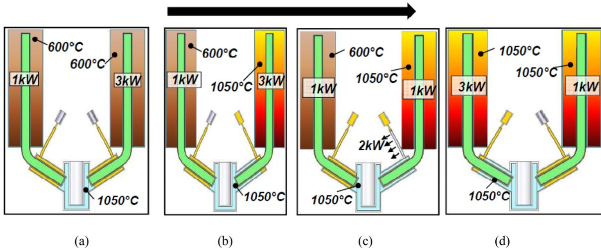
**Figure 3. The location of the gas fronts is varied to control the power into both reactors. (a) Initial Startup, (b) Move NCG front up on the right hand side to gradually heat up the cold regolith, (c) Dumping excess heat to the secondary condenser on the RHS after the RHS reactor has reached the final temperature, (d) NCG front locations while the RHS is processing, and the regolith is the LHS is heating up.**
