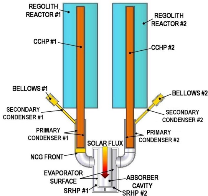
**Figure 2. PCHP (SRHP) concept for solar receiver with dual regolith reactors using bellows to vary the reservoir volume.**
