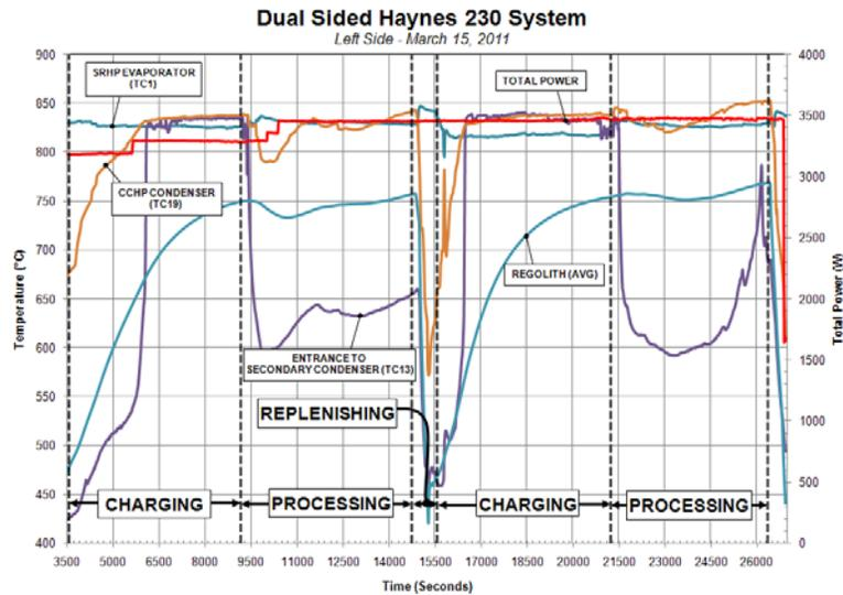
Figure 8. Dual sided Haynes 230 & sodium demonstration system - left side operation.
