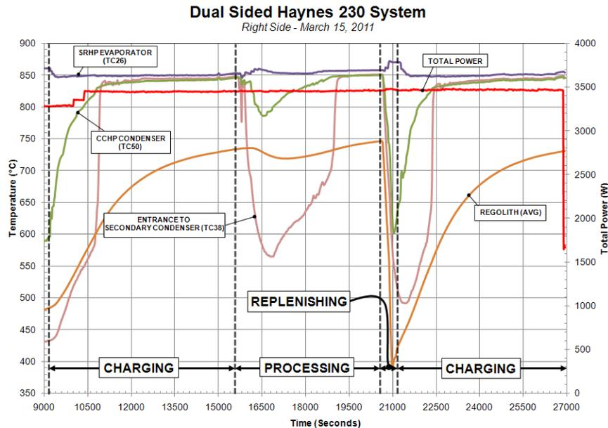
Figure 9. Dual sided Haynes 230 & sodium demonstration system - right side operation.
