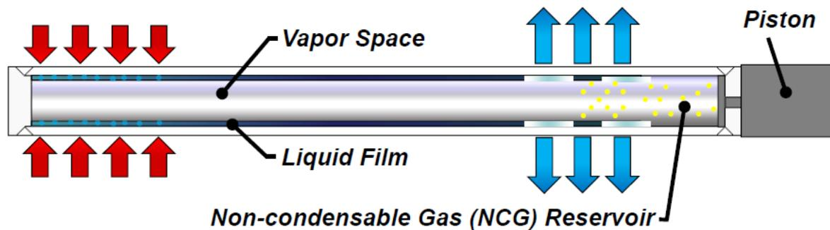
**Figure 1. Pressure Controlled Heat Pipe schematic, with the volume modulated with a piston.**
