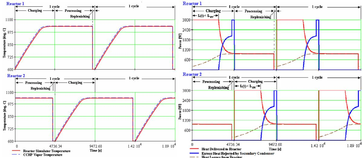
**Figure 4. Transient regolith and CCHP vapor temperatures for the two reactors during two cycles (left); Heat flow rate (Q) from SRHP to regolith for each reactor (right).**
