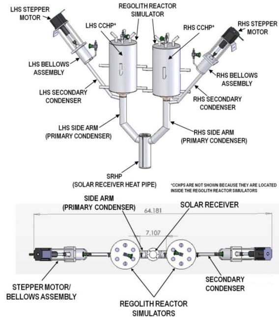
Figure 5. Final High-temperature Dual-Sided Alkali Metal/Haynes 230 system.
