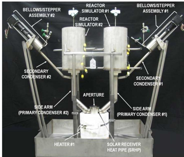
Figure 6. Dual sided Haynes 230 demonstration system test setup.
