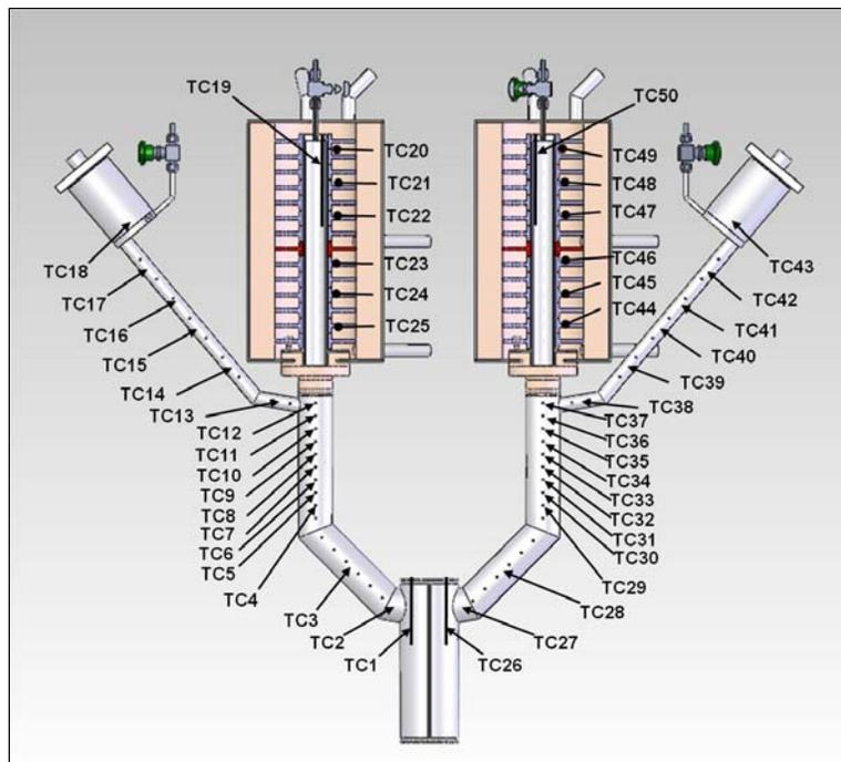
Figure 7. TC map for the dual sided Haynes 230 demonstration system.
