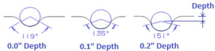
**Figure 12. Schematic showing the variation of the contact angles and depths associated with the adhesive bond geometry that were be evaluated**
