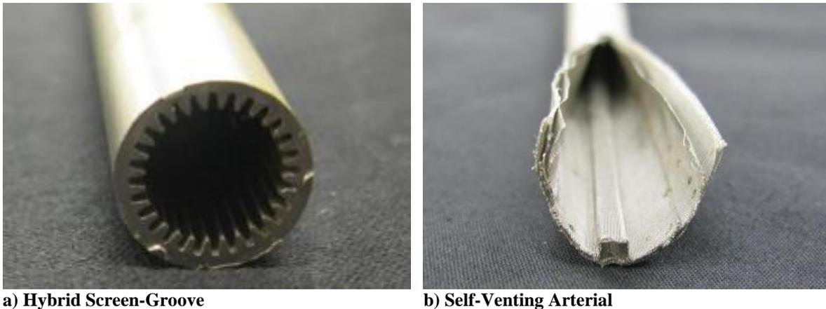
Figure 3. Heat Pipe Wick Structures Evaluated for the Kilopower Program.
