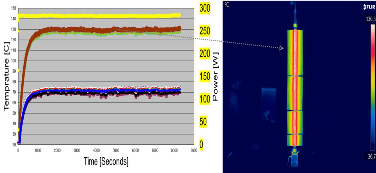
Figure 15. Thermal Image of S-Bonded Heat Pipe Radiator.
