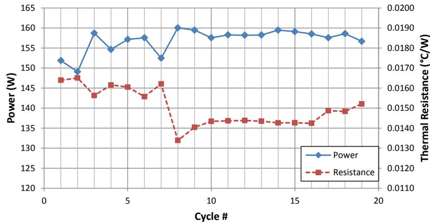
**Figure 14. Thermal Resistance History of Cycled S-Bond Heat Pipe Radiator.**
