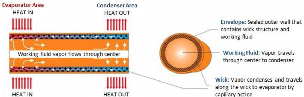
**Figure 2. Illustration of Heat Pipe Operation.**
