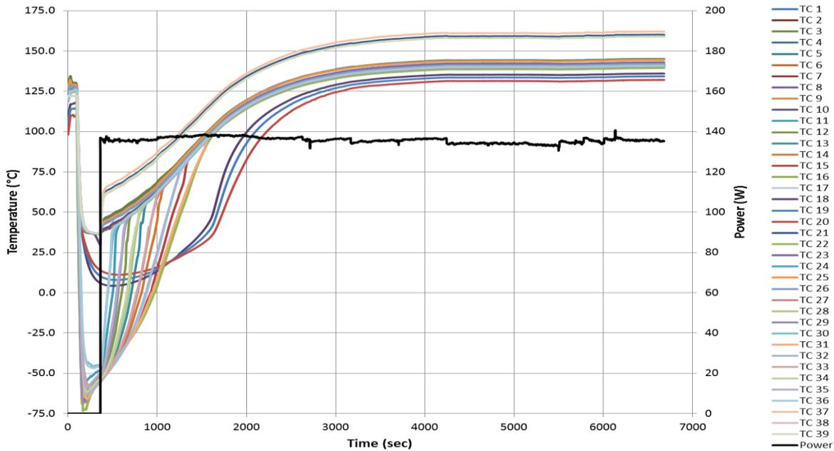
Figure 10. Freeze-Thaw Test of Hybrid Screen-Groove Heat Pipe.
