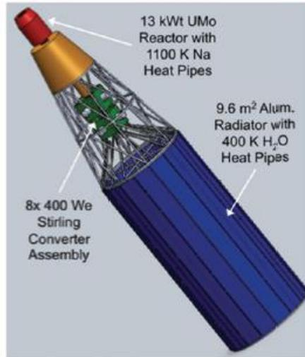
**Figure 1. Kilopower 1 kWe Design.<sup>1</sup>**
