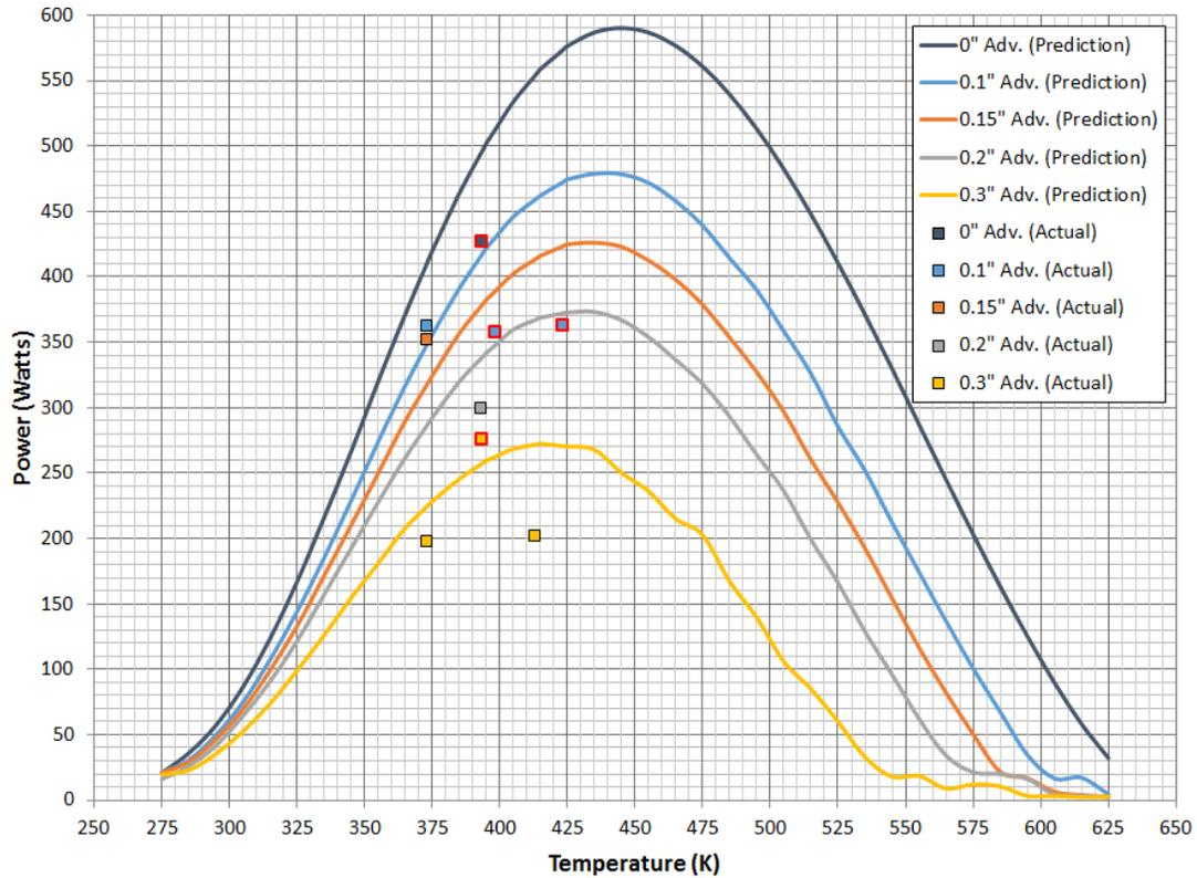
**Figure 4. Test Results vs. Predictions for Downselected Grooved Heat Pipe Design.**
