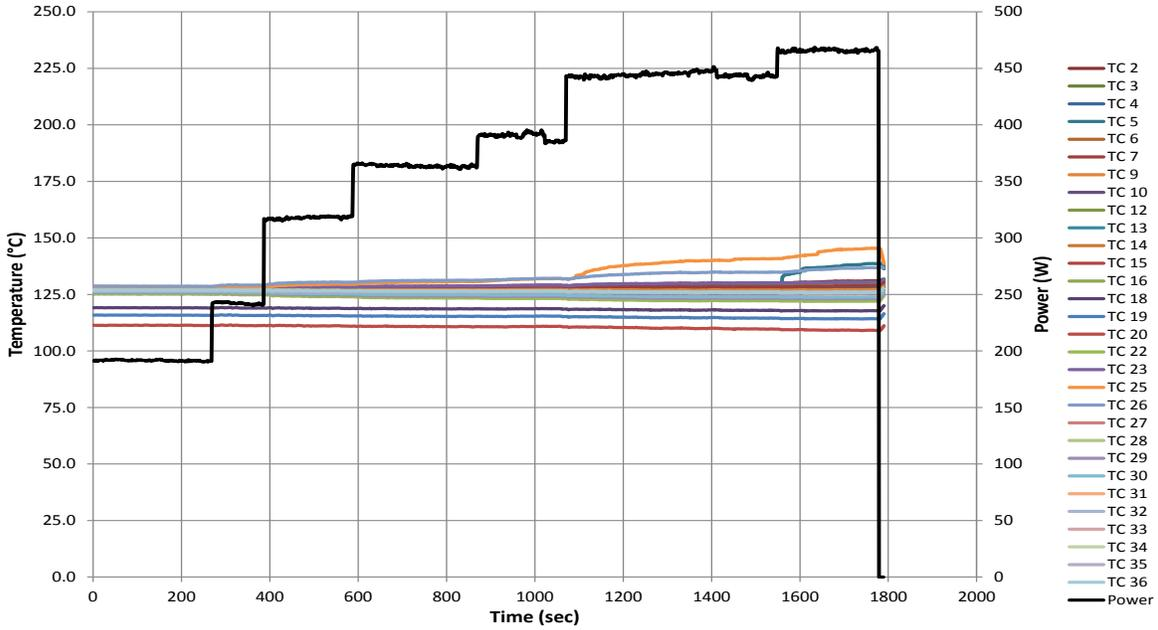
Figure 8. Performance Test of Hybrid Screen-Groove Heat Pipe.
