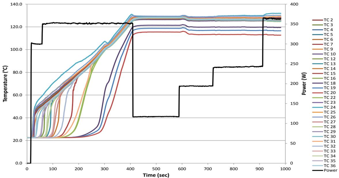
Figure 9. Vertical Orientation Test of Hybrid Screen-Groove Heat Pipe.
