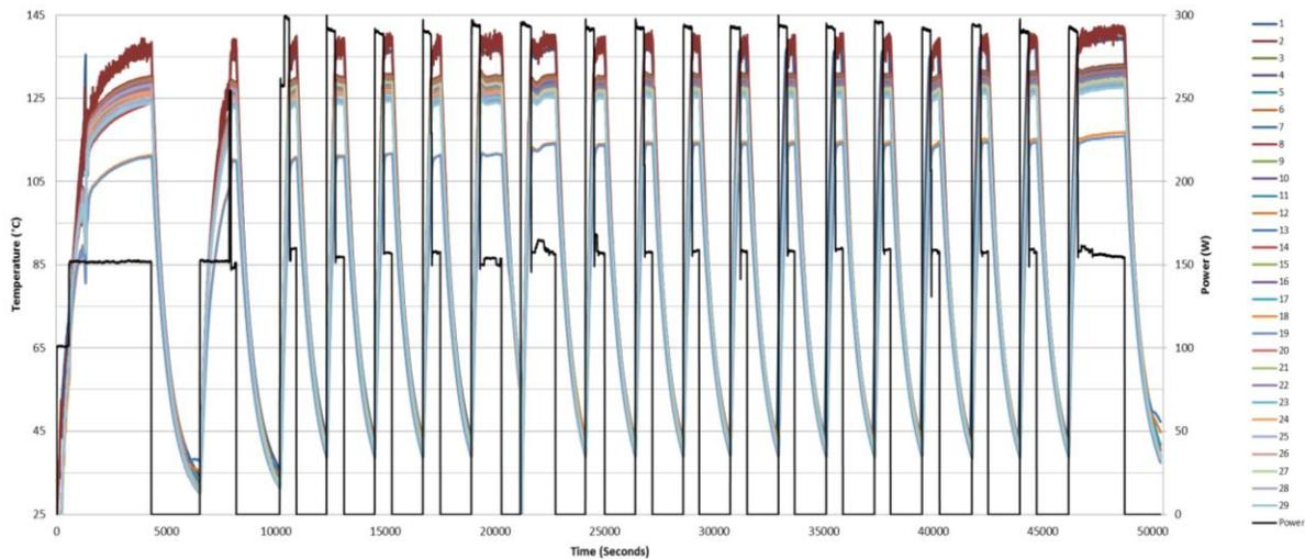
**Figure 13. Temperature Evolution of Thermal Cycle Testing of S-Bonded Heat Pipe Radiator.**
