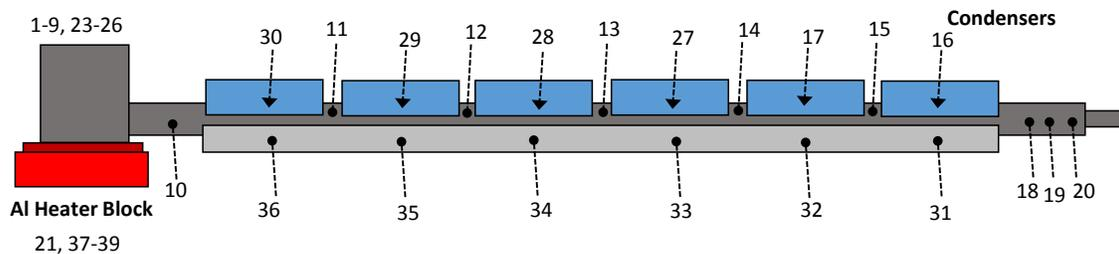
Figure 7. Thermocouple Layout for Hybrid Screen-Groove Heat Pipe.
