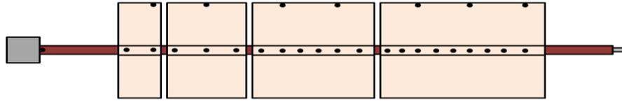
**Figure 12. Thermocouple Layout on S-Bonded Titanium - Aluminum Heat Pipe Radiator.**
