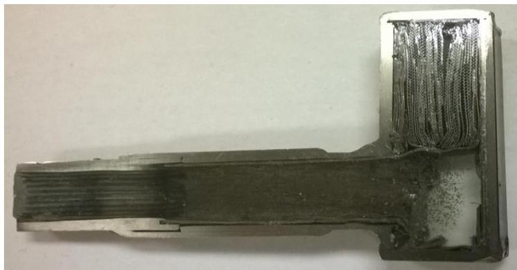
Figure 6. Cross-section of Evaporator, Accumulator, and Groove Components.
