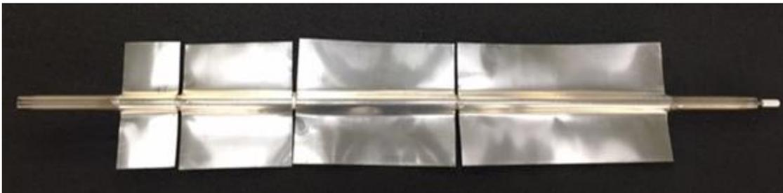
Figure 11. S-Bonded Titanium Heat Pipe to Aluminum Facesheet.
