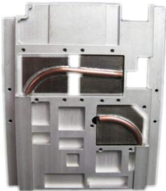
Figure 2: Standard 3U-size conduction card with integrated heat pipes. The heat pipes are able to take waste heat from chips anywhere on a board and spread it as uniformly as possible along the card edge to reduce the heat flux into the cooling rails.
