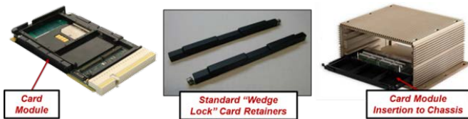
Figure 5. Typical conduction cooled card module, wedge lock, and chassis.
