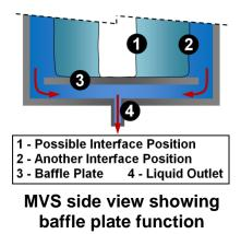
Second, a MVS does not require any moving parts. This feature provides a distinct advantage over more common vortex separation techniques, which often involve a high-speed rotating disc or separation chamber. By using a fixed chamber, complicated seals are eliminated and power requirements, failure modes, and overall device complexity are greatly reduced. This, in turn, significantly reduces fabrication costs and maintenace requirements while increasing reliability and operational lifetime.
