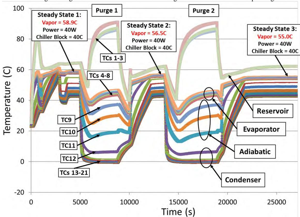
Figure 16. Example of two subsequent purge tests of the Astrobotic non-integrated hot-reservoir VCHP. Test was initiated after several days of non-operation allowing working fluid to diffuse into the NCG reservoir resulting in a higher steady-state operating temperature. During the Purge tests, power to the evaporator was turned off and 12W of heater power was applied directly to the NCG reservoir using a dedicated heater. Refer to Figure 11 for TC numbers.
