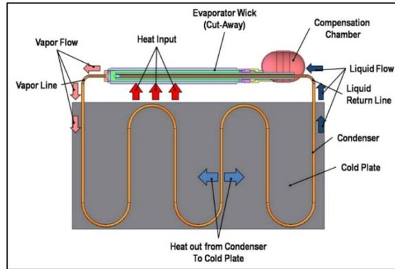
**Figure 2. Loop Heat Pipe Schematic (Not to scale).**
