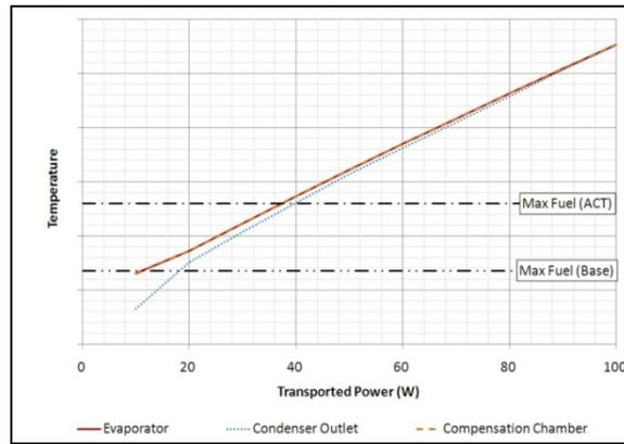
**Figure 4. LHP Temperature for Varying Power at Sink 2, Ground Conditions**
