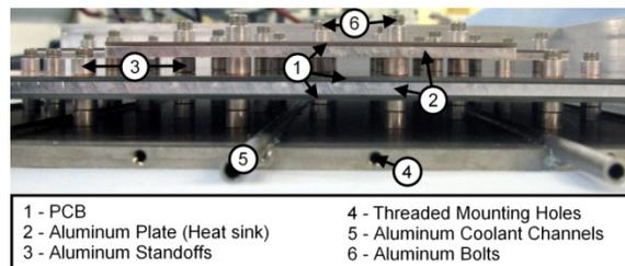
*Figure 10. Side View of Generic Avionics Test Unit*
