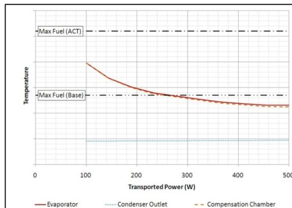
**Figure 6. Temperatures for Varying Power at Sink 2, Dash Conditions**
