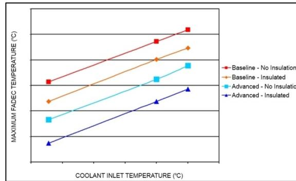
**Figure 19. Maximum Avionics Temperature for Varying Inlet Temperature and Heat Gain**
