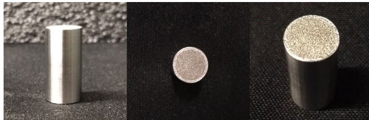
Figure 4. 3D printed wick sample used in the current study for the advancement of primary wick.
