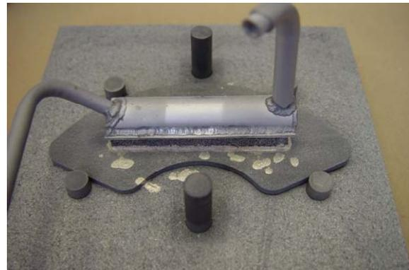
**FIGURE 10.** Photograph of the final brazed structure with 8mm thick POCO foam transition member.
