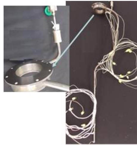
Figure 4. Kilopower heat pipe with thermocouples attached. The insert shows the annular condenser, which for this heat pipe mounts to the underside of the mounting plate.
