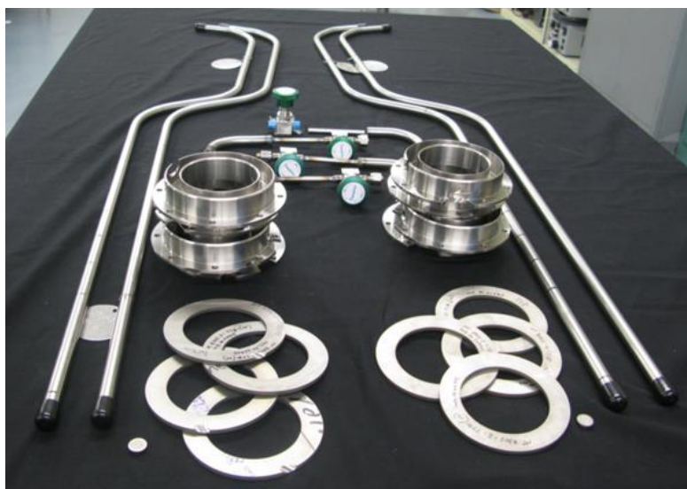
Figure 19. Remaining second generation thermosyphons ready for welding. An additional two thermosyphons are currently being tested.
