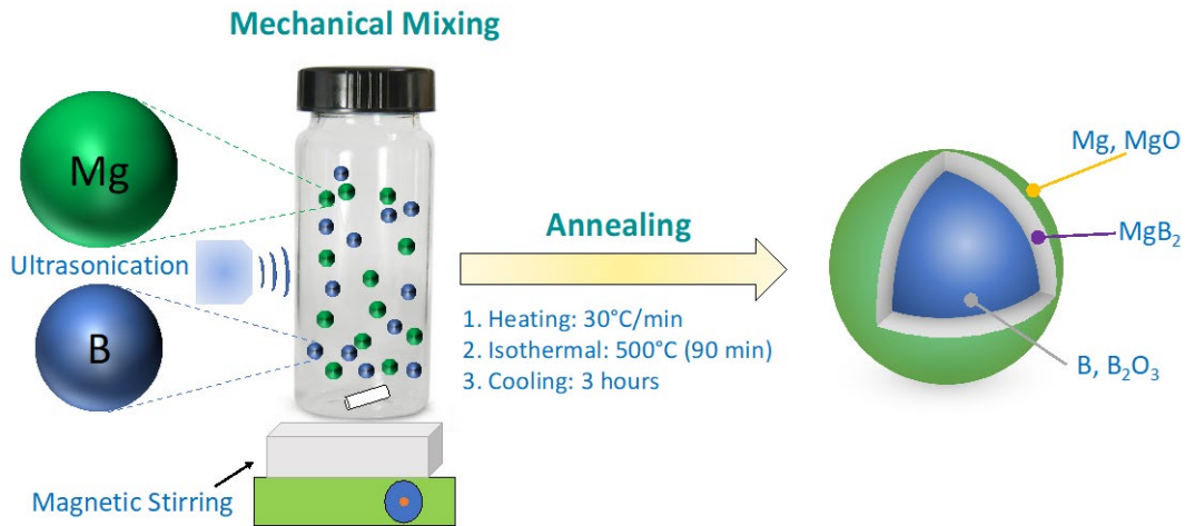
Figure 1. Schematic of the experimental method used for the synthesis of solid solutions of Mg/B.
