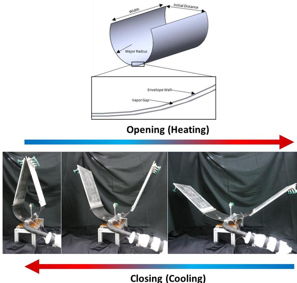
**Figure 1. Schematic of VVFTPR flexible section and images of the Phase I SBIR prototype<sup>4,5</sup>.**
