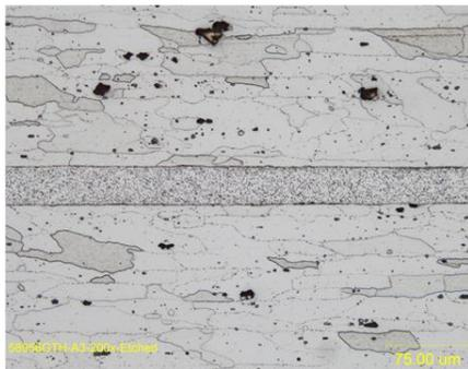
**a) 0.012 in. thick with 0.001 in. thick interlayer. Defect Free Weld.**
