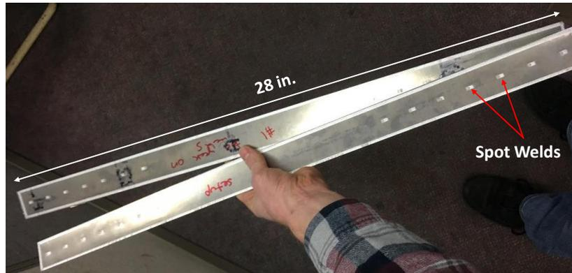
**Figure 12. Preliminary single-channel prototypes manufactured by EWI with ultrasonic welding**
