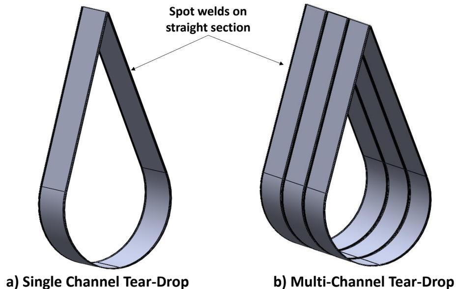
Figure 8. 3D models of preliminary VVFTPR prototype
