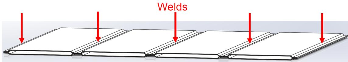
Figure 6. Welding pattern for multi-channel VVFTPR
