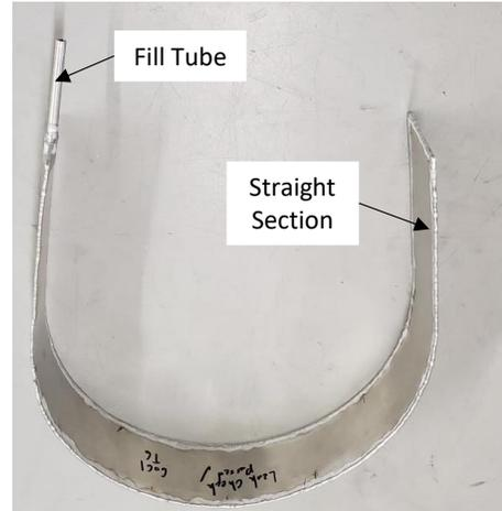
**Figure 3. Small prototype strip for pressure testing. Aluminum 6061.**
