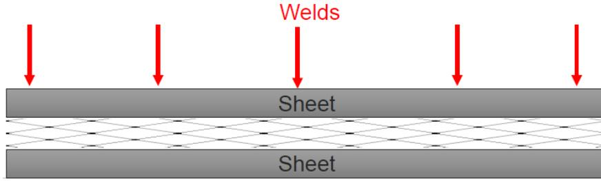
Figure 7. Setup of envelope material and screen wick for welding.
