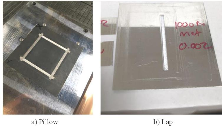
**Figure 10. Weld configurations used for iterative weld development testing.**
