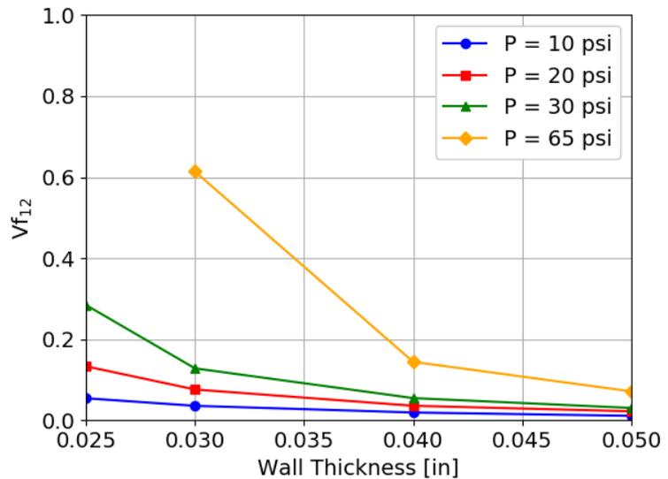
**Figure 8.** Effect of wall thickness on the view factor  $V_{f,12}$ .  $R = 4.0$  in.,  $\theta = 90^\circ$ , vapor space gap = 0.02 in., channel width = 2.0 in.,  $Z = 12.0$  in.
