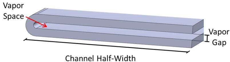
**Figure 4. Geometry of the modular channel used for 3D simulations.**
