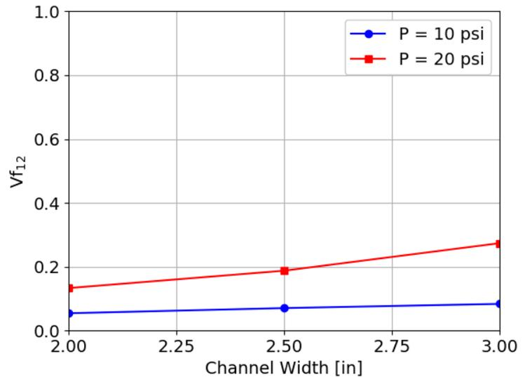
**Figure 6. Effect of channel width on the view factor  $V_{f,12}$ .  $R = 4.0$  in.,  $\theta = 90^\circ$ , wall thickness = 0.025 in., vapor space gap = 0.02 in.,  $Z = 12.0$  in.**
