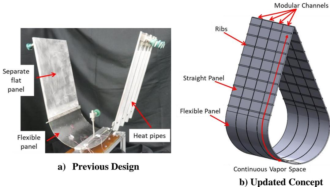
**Figure 2. Overview of previous design concept and the updated design concept for the variable-view factor two-phase radiator.**
