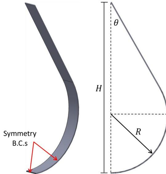
**Figure 3. 3D Model for simulations and relevant geometric variables.**
