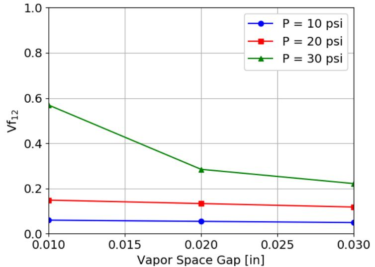
**Figure 7.** Effect of vapor space gap on the view factor  $V_{f,12}$ .  $R = 4.0$  in.,  $\theta = 90^\circ$ , wall thickness = 0.025 in., channel width = 2.0 in.,  $Z = 12.0$  in.
