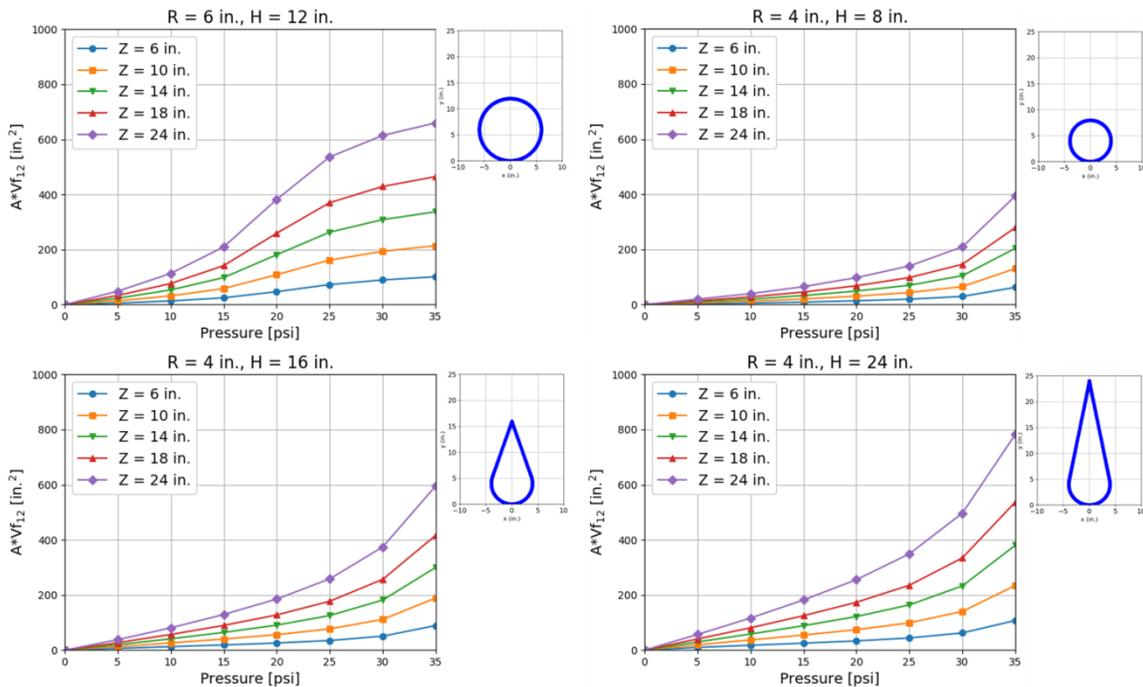
**Figure 10. Effective Area ( $AV_{f,12}$ ) of the four profiles as functions of internal pressure and radiator depth  $Z$ . Wall thickness = 0.025 in., channel width = 2.0 in. and vapor space gap = 0.02 in.**
