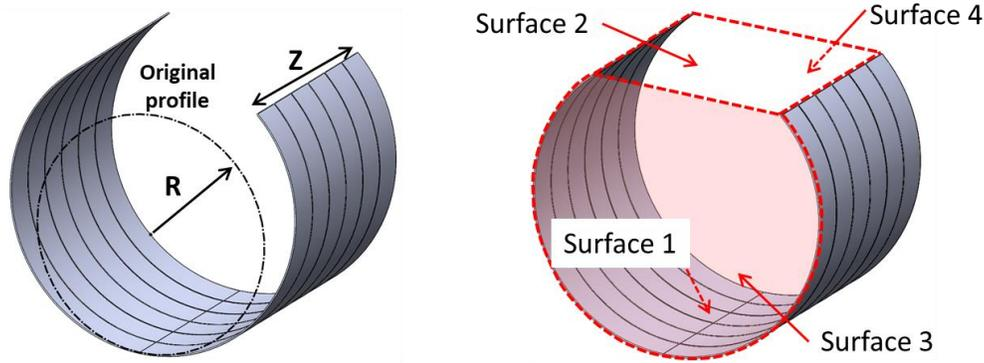
**Figure 5 Surfaces used for view factor calculation.**
