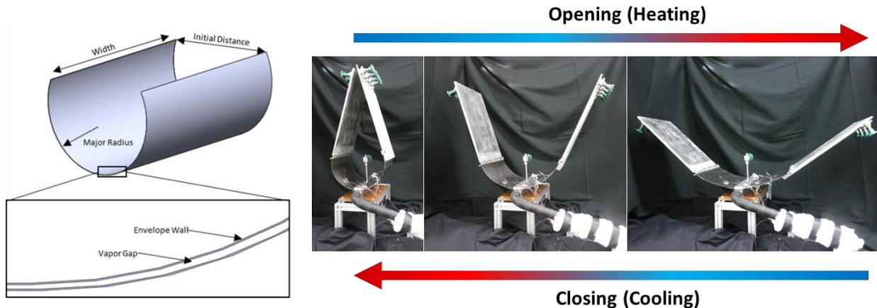
**Figure 1. Schematic of VVFTPR flexible section and images of the Phase I prototype.**
