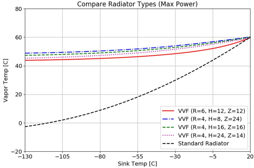
**Figure 11. Variation in vapor temperature with sink temperature for the radiator geometries listed in Table 1. A “Standard Radiator” represents a flat radiator ( $V_{f,12} = 1$ ) sized to dissipate max power at max sink temperature. Max Power = 40 W.**
