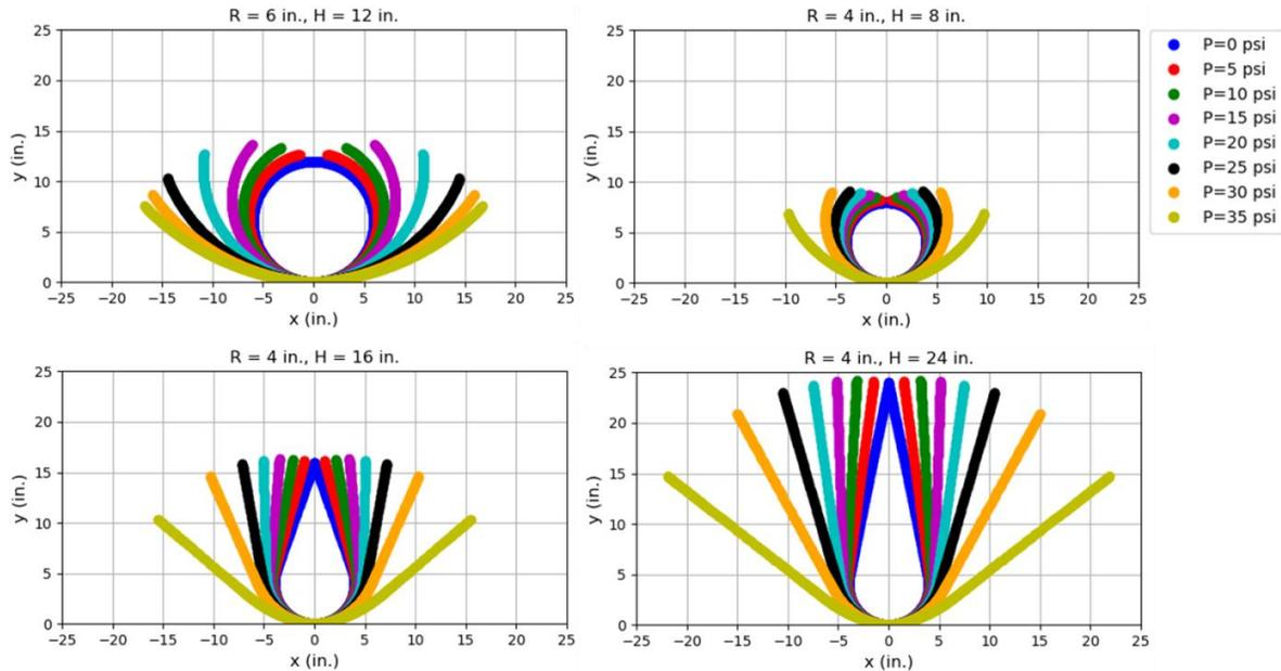
**Figure 9. Effect of pressure on the shape of the VVFTPR for several profile shapes. Wall thickness = 0.025 in., channel width = 2.0 in. and vapor space gap = 0.02 in.**
