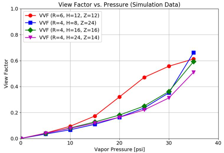
**Figure 12. Variation in view factor  $V_{f,12}$  with vapor pressure for the 4 profiles listed in Table 1.**
