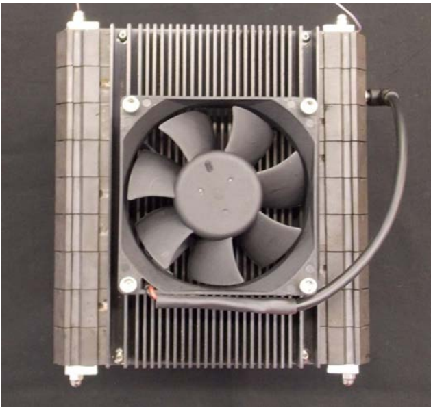
Figure 7. External Finstack and Fan attached over the Exposed Through-wall Heat Pipes of the CFRP Enclosure
