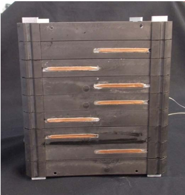
Figure 6. Assembled CFRP Enclosure Slices with Exposed Copper Heat Pipe Sections prior to Attaching the External Finstack
