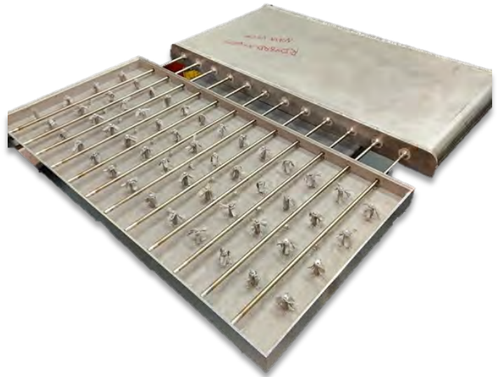
Figure 10. Full-Scale VCCP. The lid of the Vapor Chamber is removed in this image to provide an interior view.
